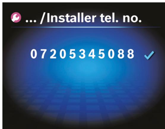
Telephone number can be added to the control display for easy contact and resolution.
