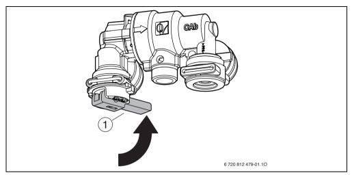
Fig. 11 Stop filling the heating system
