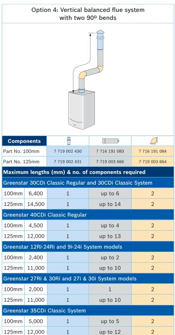
**Note:** The 100mm dia. short flue extension (Part No. 7 716 191 133) and 100mm dia. 2m flue extension (Part No. 7 716 191 172) may be used as an alternative to the standard extension as required up to the maximum flue lengths stated.
