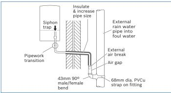
Fig. 4 Disposal into a rainwater down pipe
