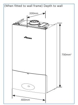
Greenstar 9i-24i System †710mm to top of casing front.
