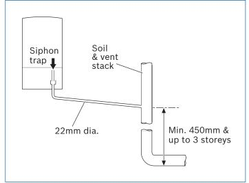
Fig. 1 Disposal to soil vent stack
