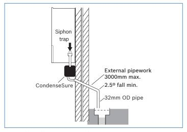
A typical installation using CondenseSure
