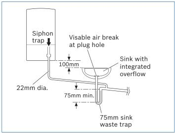
Fig. 2 Disposal to a waste pipe
