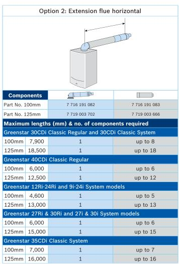
**Note:** The 100mm dia. short flue extension (Part No. 7 716 191 133) and 100mm dia. 2m flue extension (Part No. 7 716 191 172) may be used as an alternative to the standard extension as required up to the maximum flue lengths stated.
