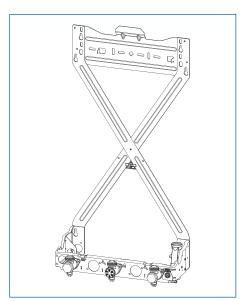
Greenstar 9i-24i System boiler wall-mounting jig
