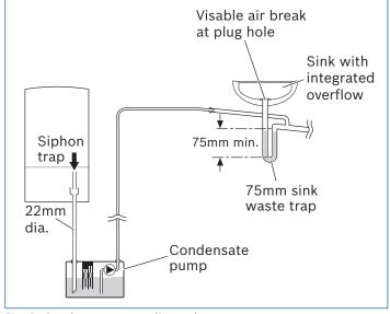
Fig. 3 Condensate pump disposal
