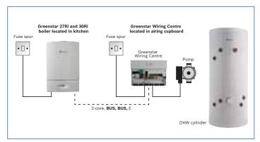
System layout with a Greenstar Wiring Centre
