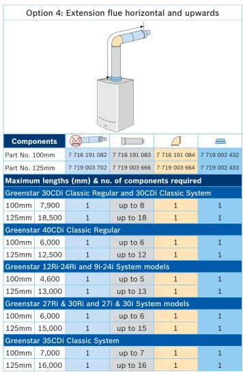
**Note:** The 100mm dia. short flue extension (Part No. 7 716 191 133) and 100mm dia. 2m flue extension (Part No. 7 716 191 172) may be used as an alternative to the standard extension as required up to the maximum flue lengths stated.
