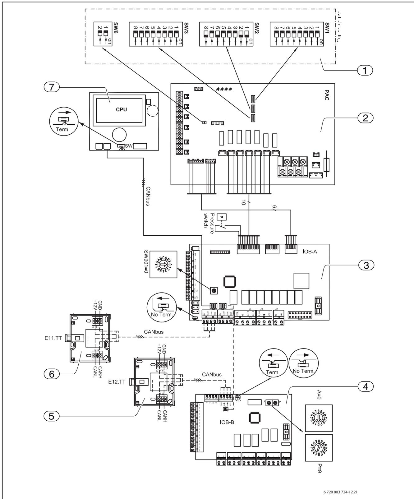
Fig. 38 Switch settings for Hydrolight unit with additional mixed heating circuit (accessory)
