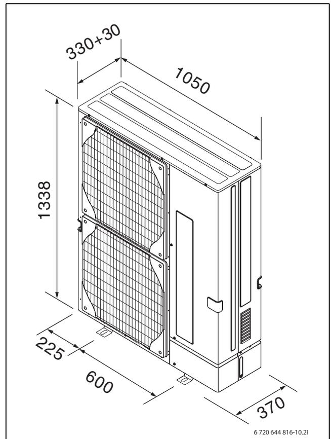
Fig. 11 ODU 10, 11 and ODU 12, dimensions in mm
