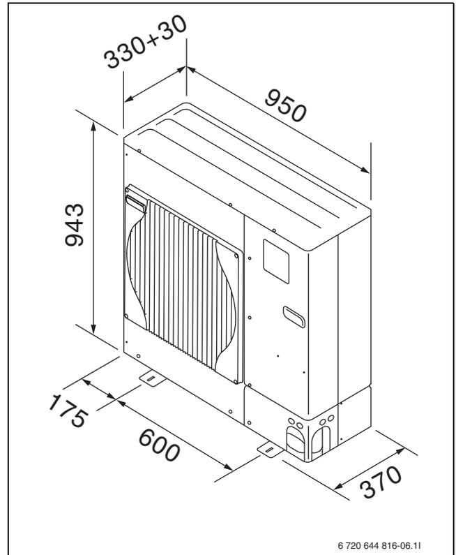
Fig. 10 ODU 7.5, dimensions in mm
