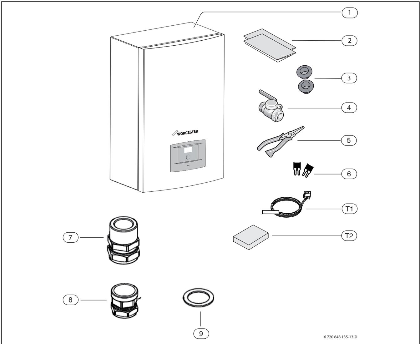
Fig. 2 Standard delivery, Hydrolight/Hydrocomfort 16 module
