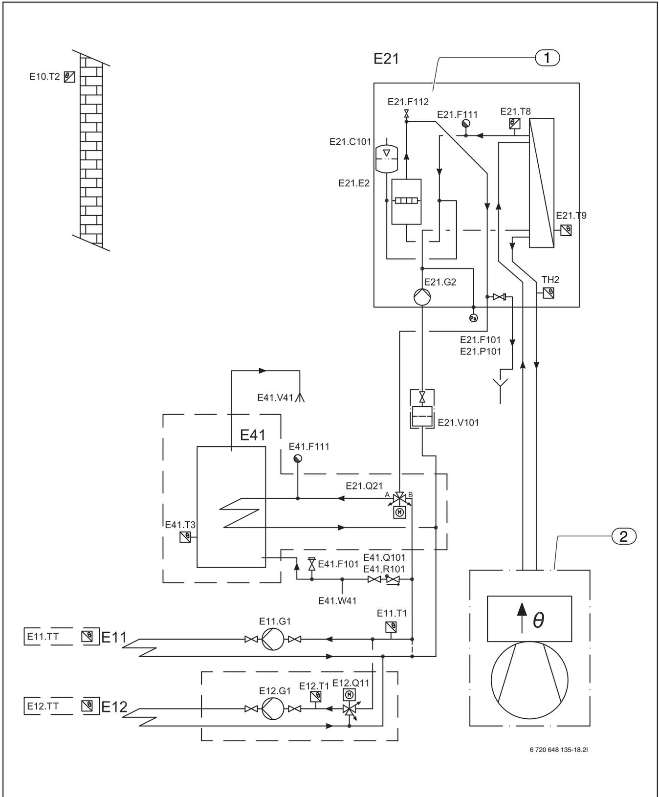
Fig. 53 Hydrocomfort with DHW cylinder and central heating
