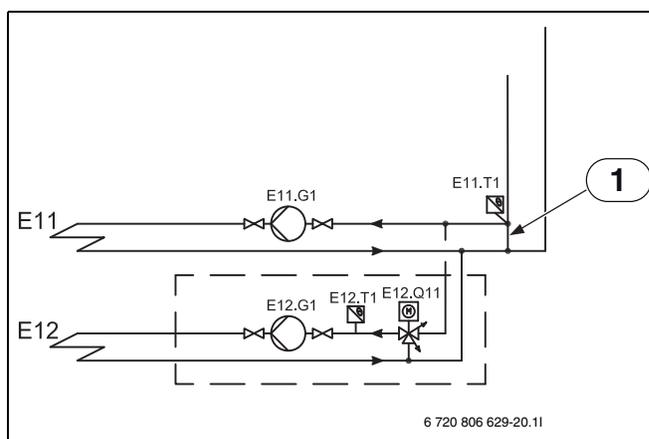
Fig. 52 Additional mixed heating circuit
