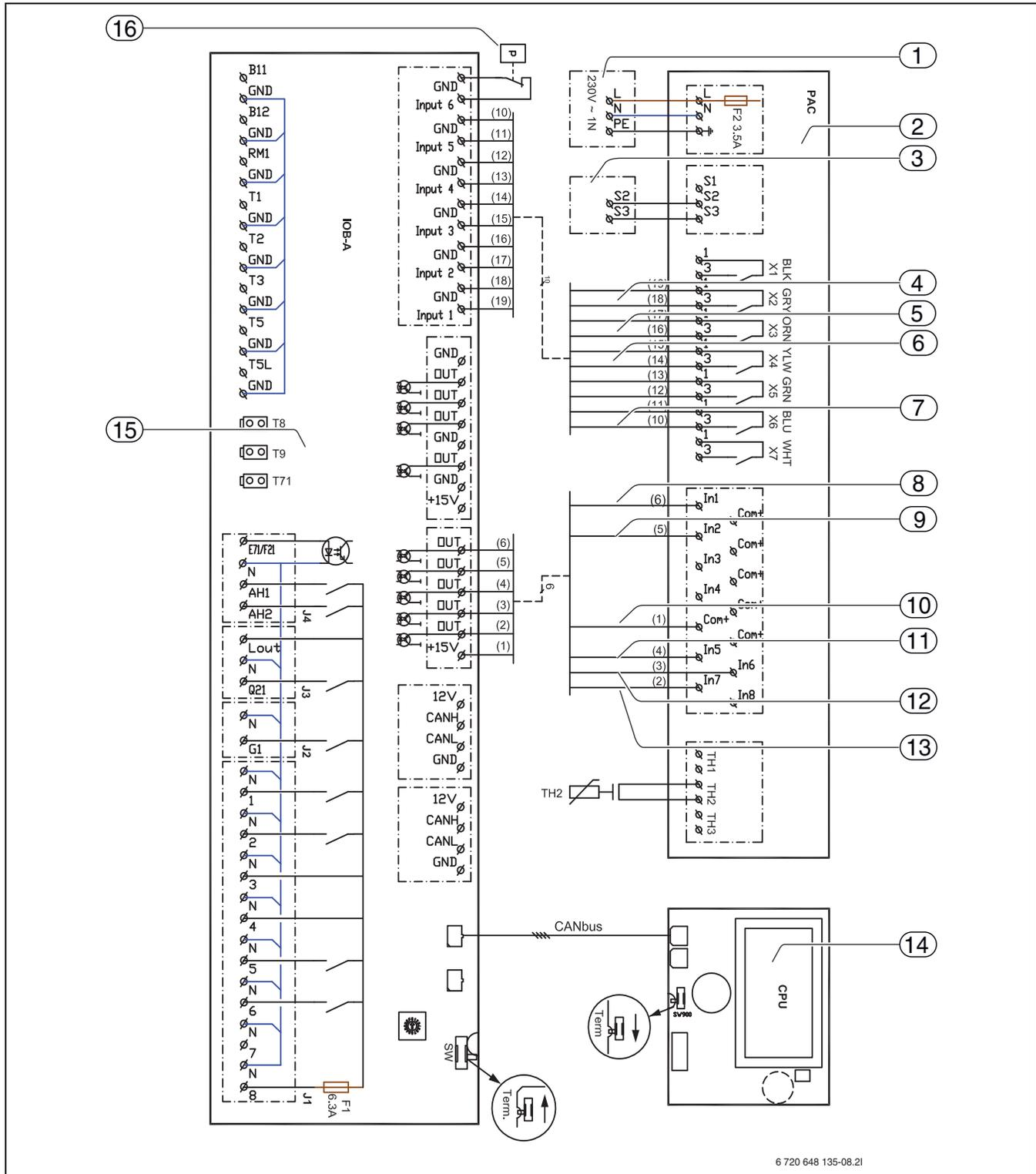
Fig. 48 Signal cable, Hydrocomfort unit with electr. heater
