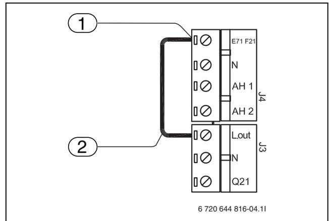
Fig. 35 In-coming alarm signal from mixed additional heat
