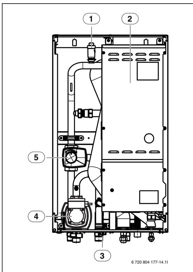
Fig. 23 Hydrolight unit with mixing valve for 2. heat appliance
