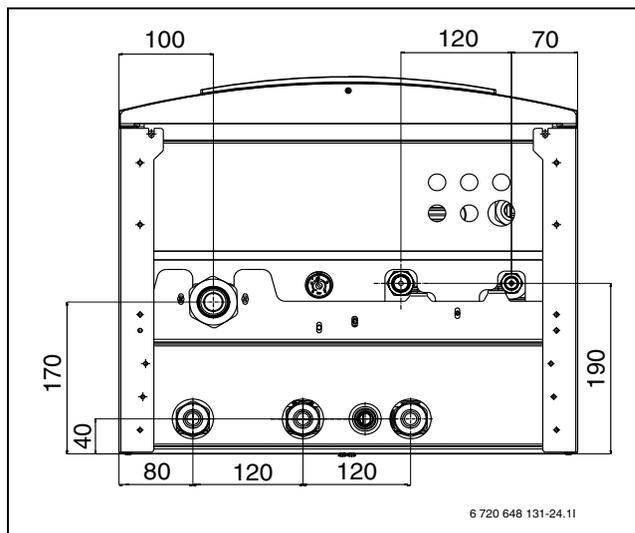
Fig. 15 Pipe connections of dual mode Hydrolight unit, with mixing valve for 2. heat appliance.
