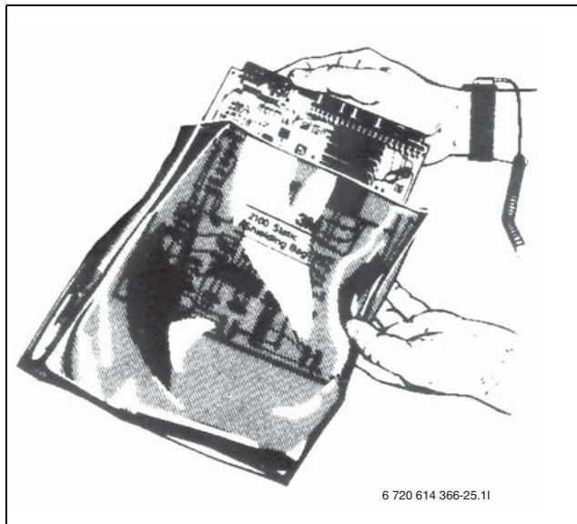
Fig. 7 Using an anti static bracelet
