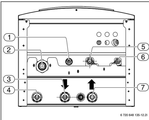
Fig. 17 Pipe connections of dual mode Hydrolight unit, with mixing valve for 2. heat appliance.
