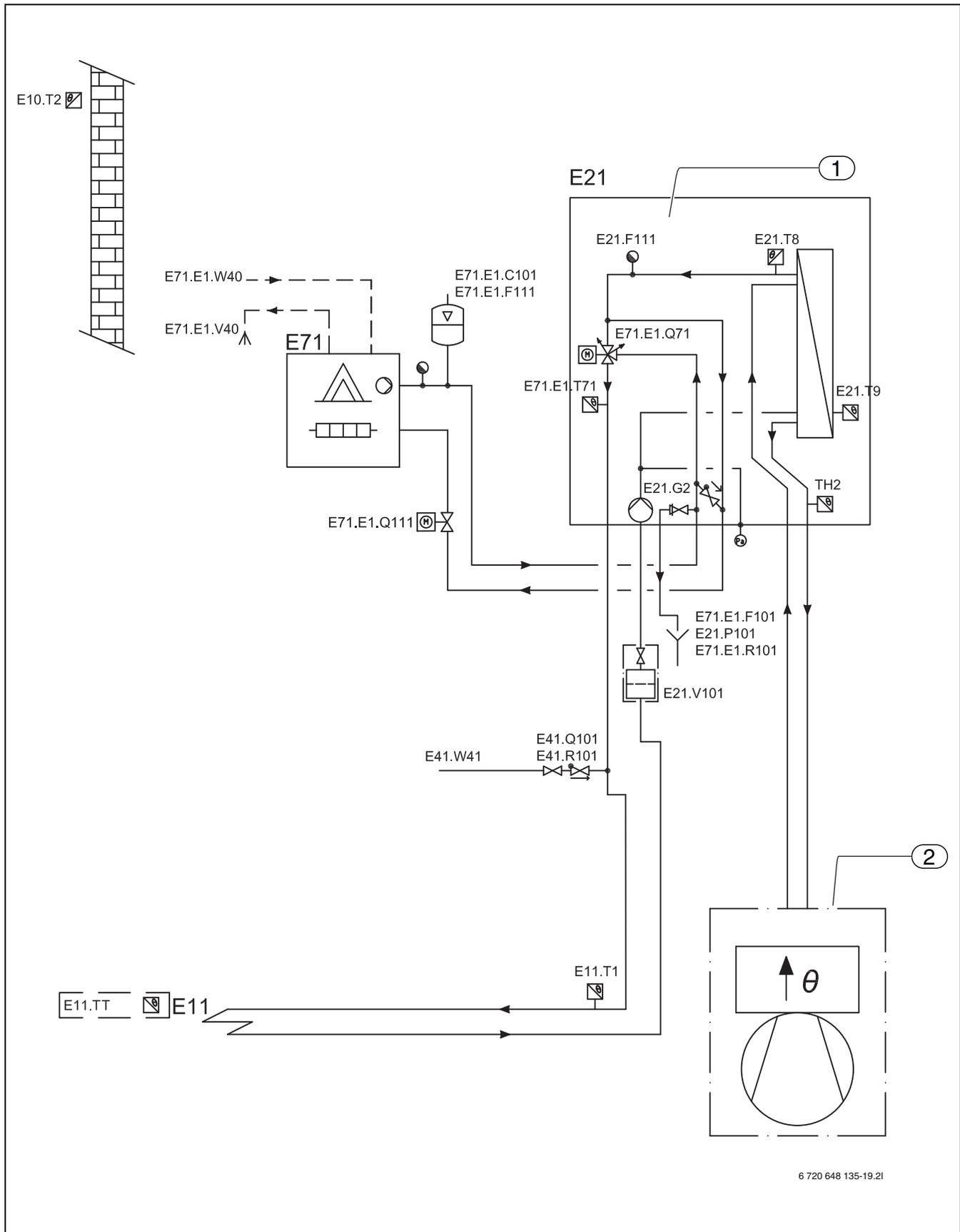
Fig. 54 Additional external heater with mixer
