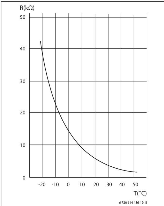
Fig. 58 Low-temperature sensor ODU
