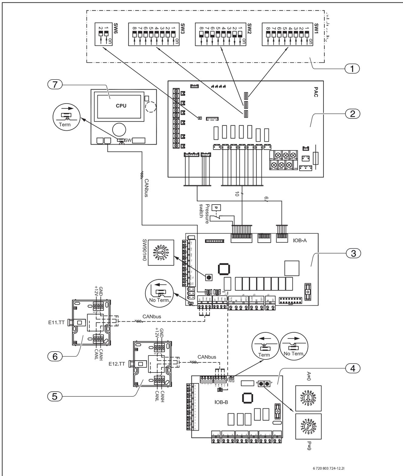
Fig. 44 Switch settings, Hydrocomfort module with electr. unit heater and additional mixed heating circuit (accessory)
