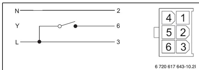
Fig. 29 Connections in Molex plug
