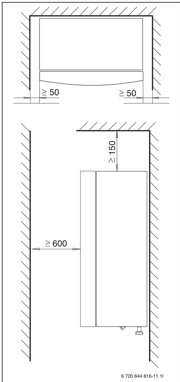
Fig. 14 Minimum dimensions of Hydrolight/Hydrocomfort unit (dimensions in mm)
