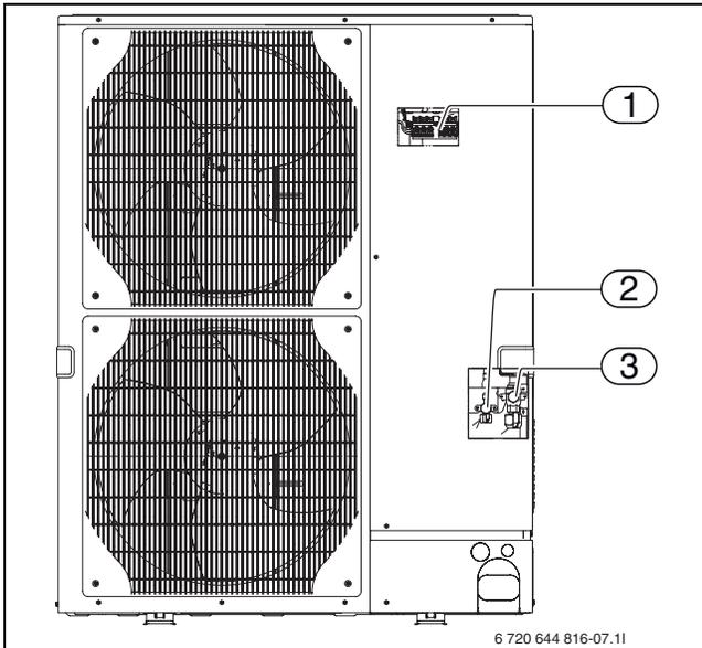
Fig. 8 Connections, outdoor unit
