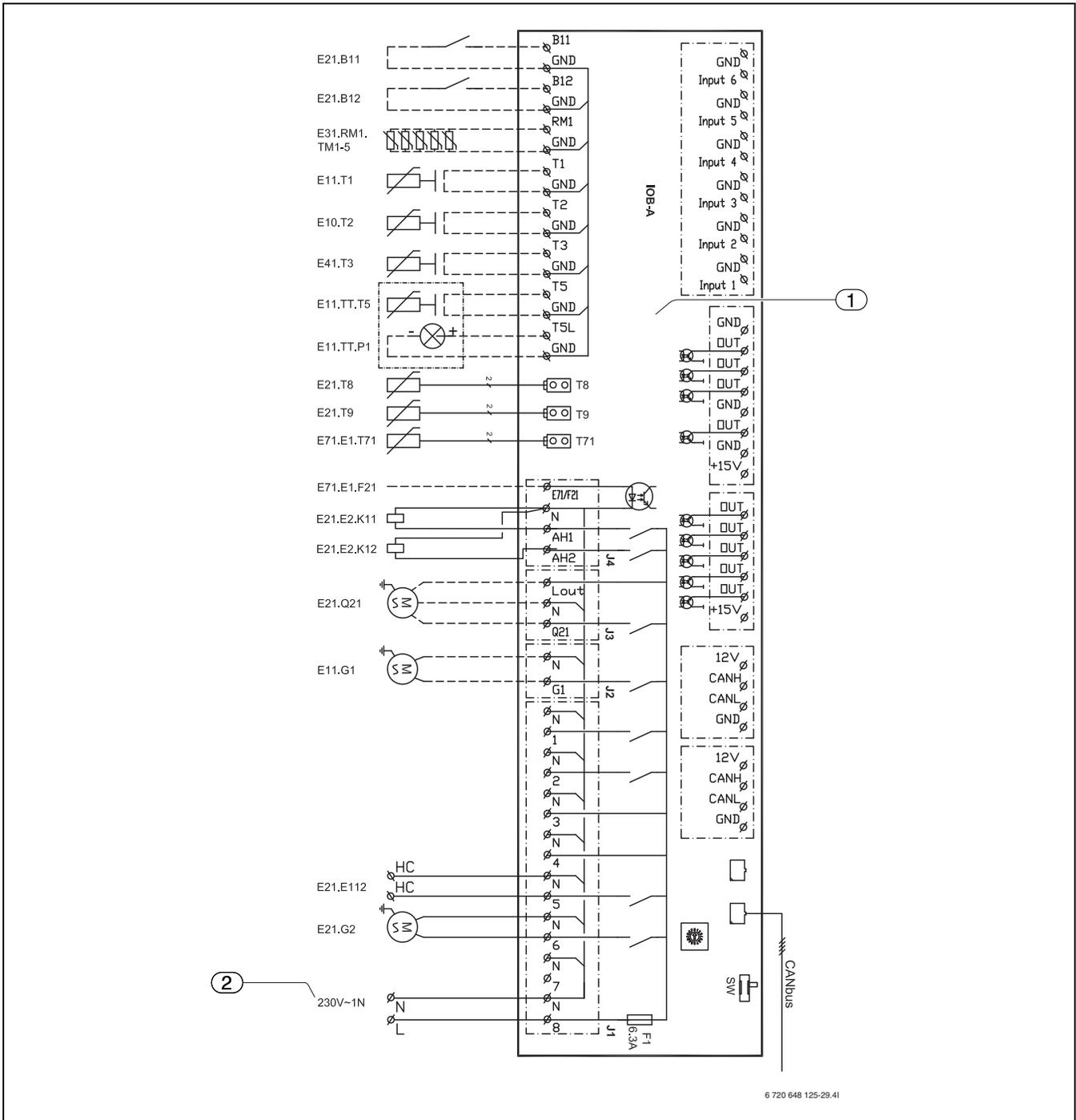
Fig. 47 Wiring diagram, Hydrocomfort unit with electr. heater
