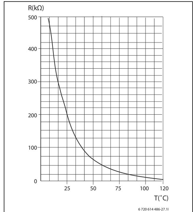
Fig. 60 High temperature sensor ODU
