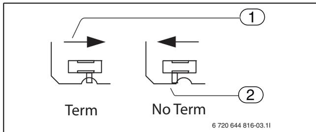
Fig. 5 CAN-BUS termination
