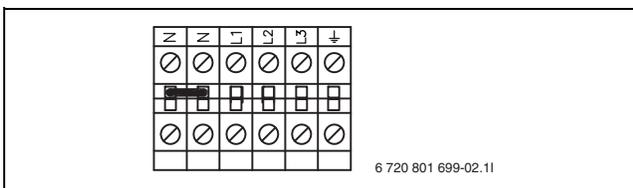
Fig. 33 Jumper position in Hydrocomfort at delivery, 3-phase
