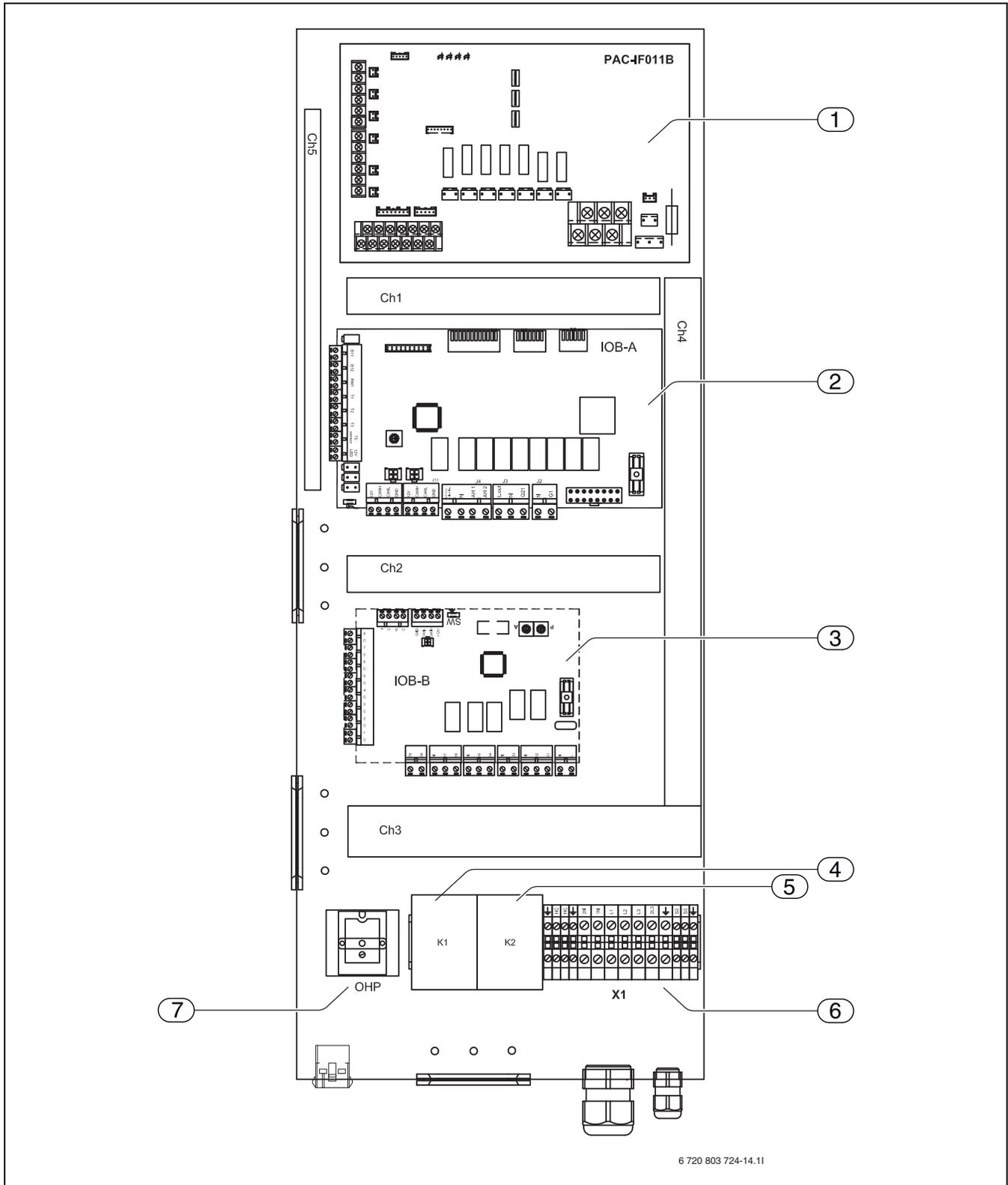
Fig. 43 Layout in control panel, Hydrocomfort unit with electr. heater
