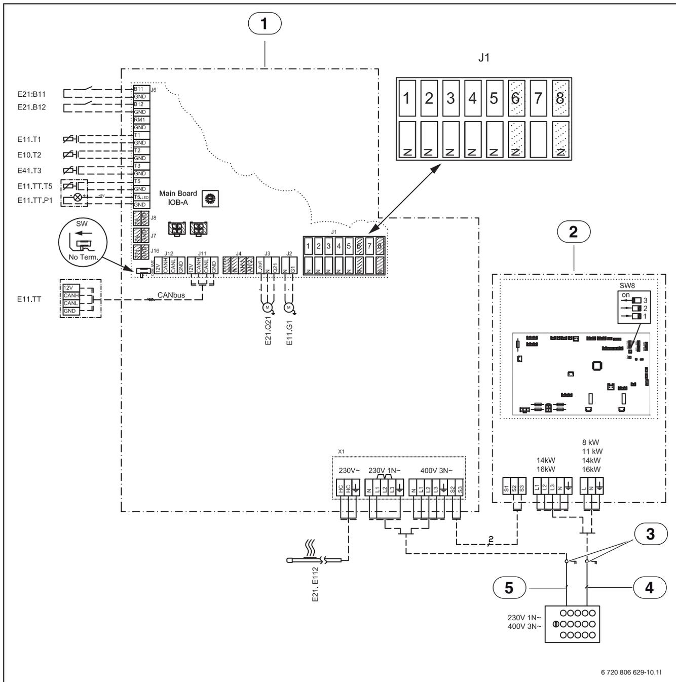
Fig. 46 Terminal connection diagram, Hydrocomfort unit with electr. heater
