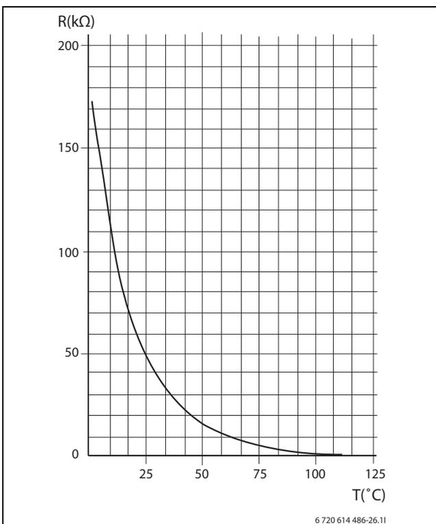
Fig. 59 Mean temperature sensor ODU
