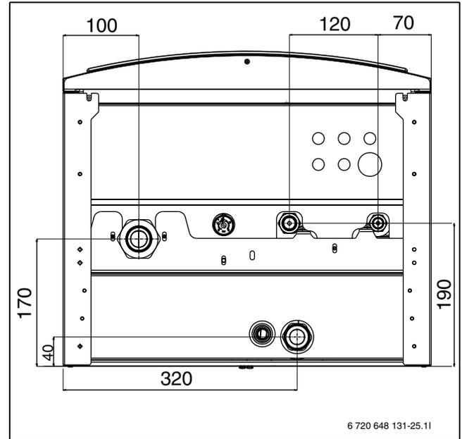
Fig. 18 Pipe connections for Hydrocomfort module with electric booster heater.
