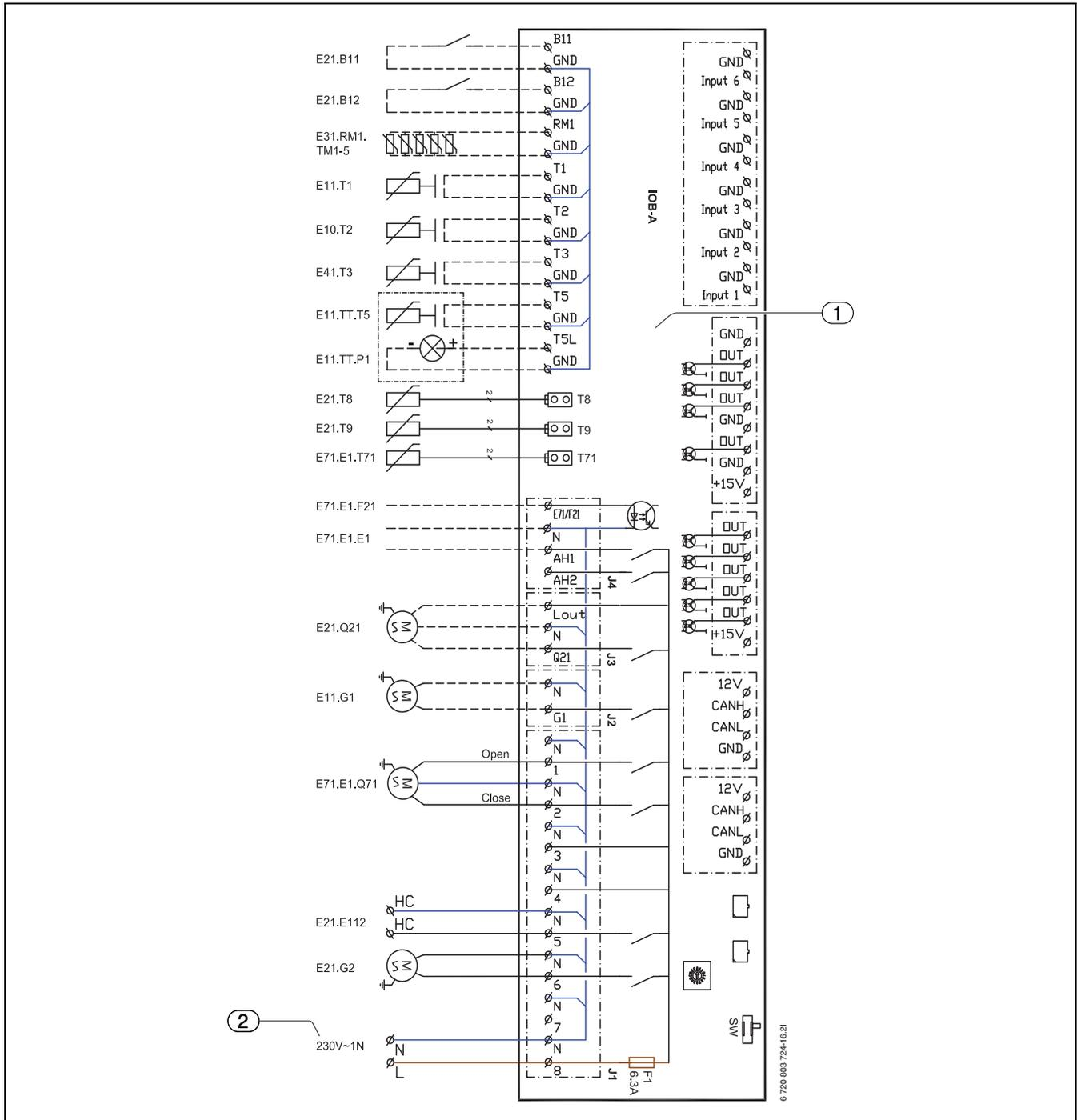
Fig. 41 Wiring diagram, Hydrolight unit with 2nd heat appliance
