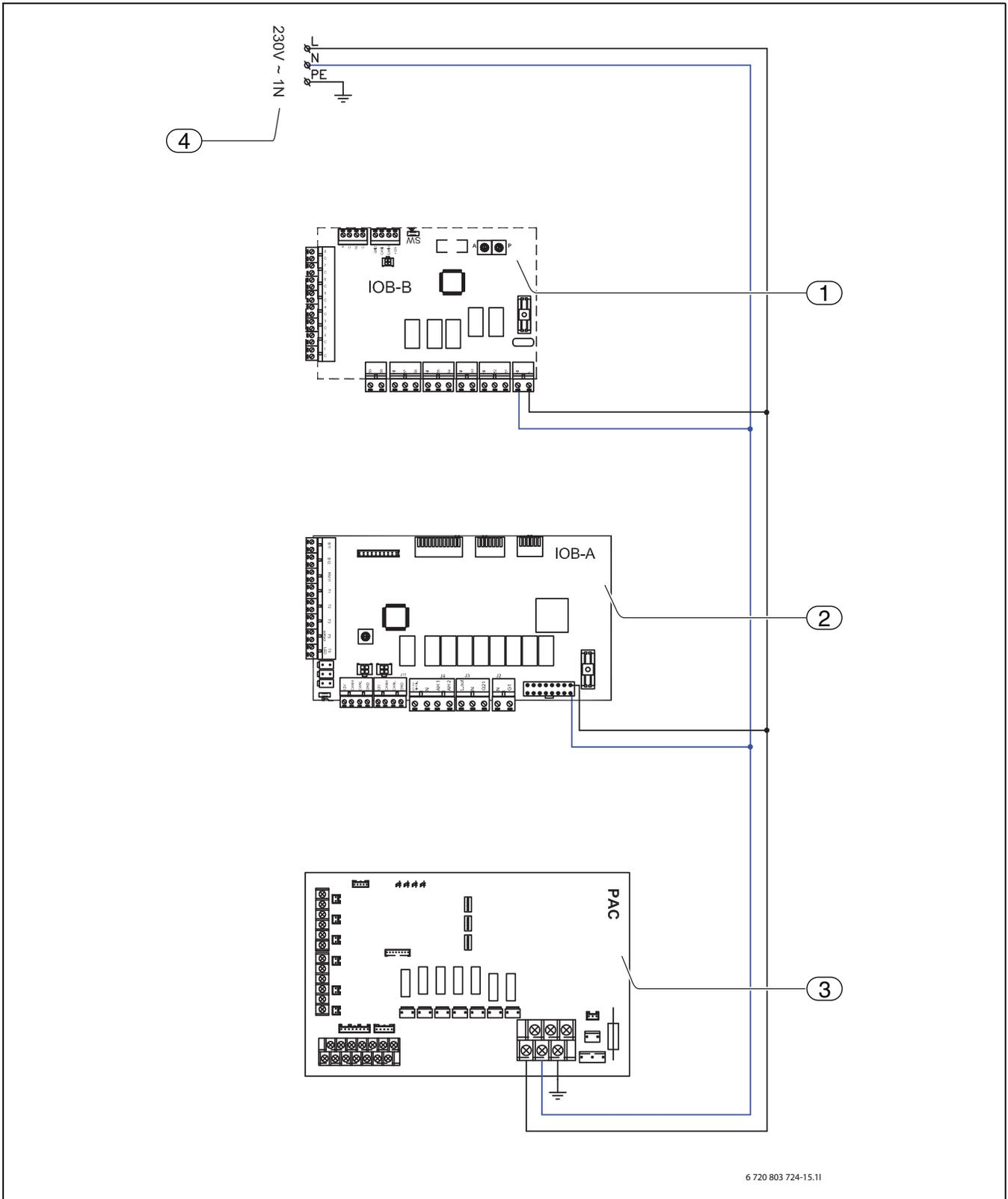
*Fig. 39 Power supply, Hydrolight unit and additional mixed heating circuit (accessory)*
