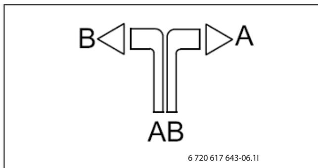
Fig. 26 Flow direction of 3-way valve
