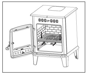
4. Slide the log retainer down into the slots located at the front of the door
