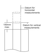
The datum for vertical measurements is the point of discharge of the flue, or 150mm above the insulation, whichever is the lower
