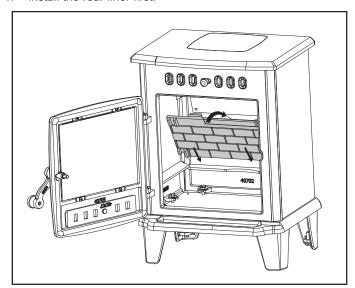
2. Next install the grate. Note that there are two small notches and two large notches. The two large notches must face to the front of the stove or the grate will not correctly install.
