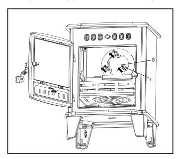
Reach in through the front door of the stove and remove the three (B) bolts, and (C) washers, that are holding on the flue collar.
