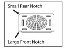
3. Install the left and right brick liners (flip left brick liner to fit).
