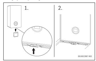
Fig. 5 Position of Key housing
