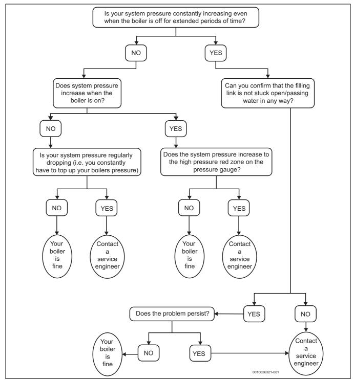
Fig. 8 Gassing flow chart
