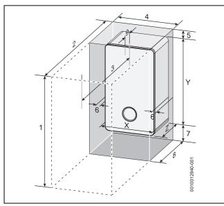
Fig. 7 Appliance minimum clearances
