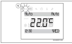
Fig. 16 Low batteries display
