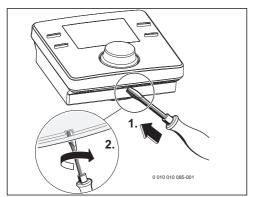
Fig. 7 Releasing control unit from wall socket
