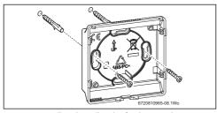
Fig. 8 Installing the wall socket for the control unit
