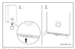
Fig. 3 Install Key
