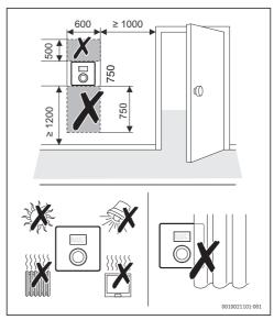
Fig. 5 Installation location of the control unit
