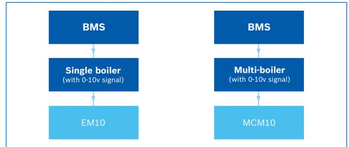
Fig. 1. Compatible BMS controls
