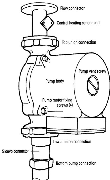
**Fig. 41. Expansion vessel and pump assembly.**
