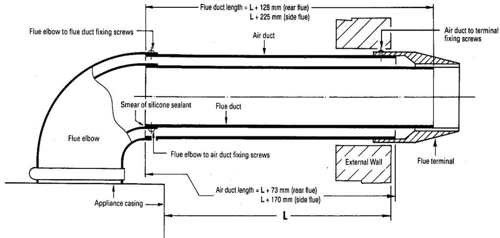
**Fig. 22. Flue assembly using the extension ducts.**
