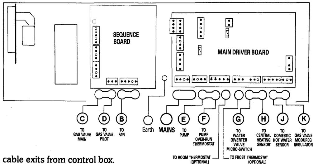
Fig. 27. Electrical cable exits from control box.
