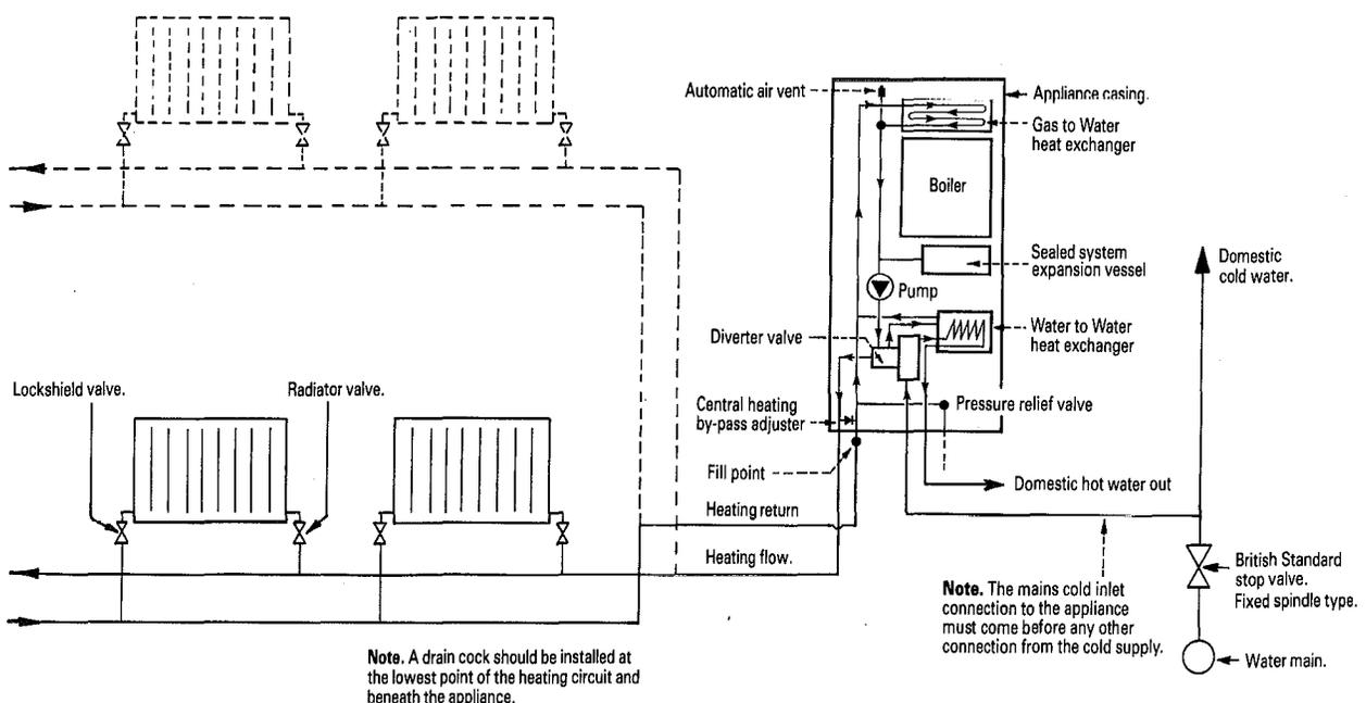
**Fig. 6. System filling and make-up.**
