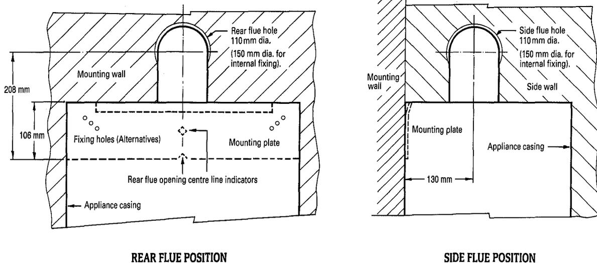
**Fig. 14. Marking out the side flue position.**
