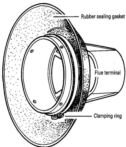
**Fig. 25. Duct and terminal assembly for internal fitting of the flue.**
