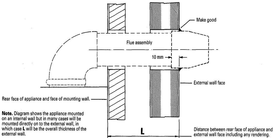
Fig. 20. Flue duct length (side flue).
