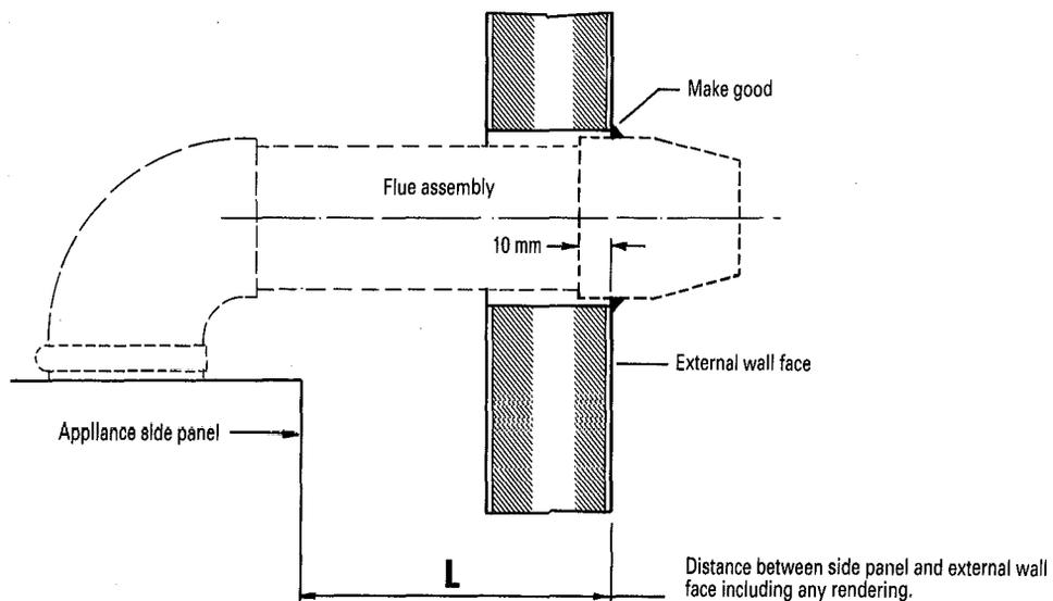
**Fig. 21. Flue elbow, ducts and terminal assembly.**
