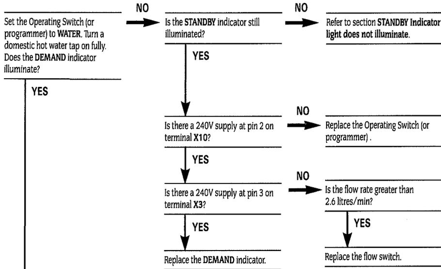
FAILURE AT POINT L
