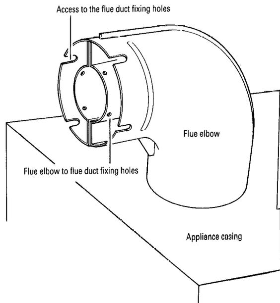
Assemble the air and flue ducts to the terminal. Drill through the holes in the terminal into the air duct and fix using the screws provided. See Fig. 21. Join the extension ducts to the standard ducts as indicated in Fig. 22 applying a smear of silicone sealant to the end of the flue duct. Drill and screw together the air ducts. From outside, push the assembly through the wall and enter the ducts into the flue outlet elbow.
