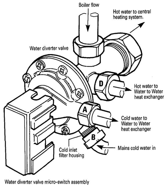
Fig. 43. Water to Water heat exchanger connections.
