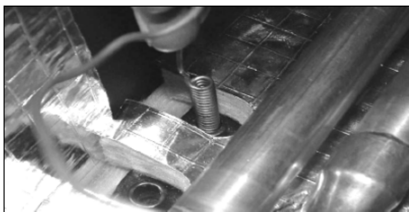
LOCATION OF LIMIT THERMOSTAT PHIAL
