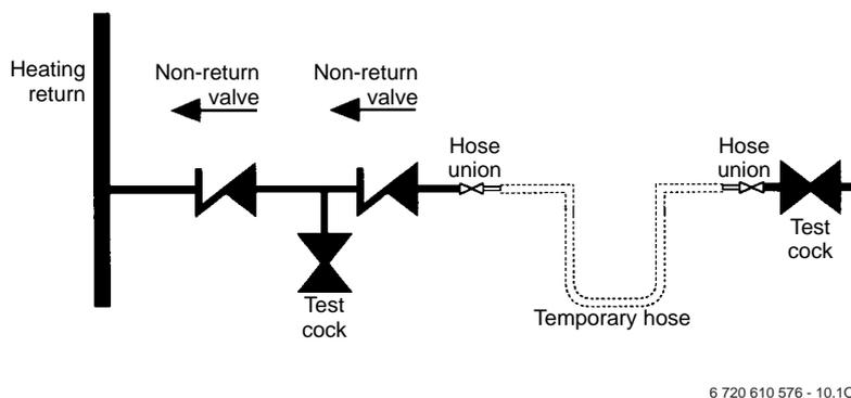
Fig. 6 Sealed primary water system - filling method
