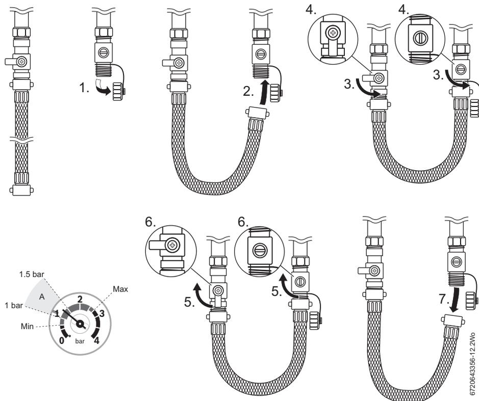
Fig. 7 External filling loop
