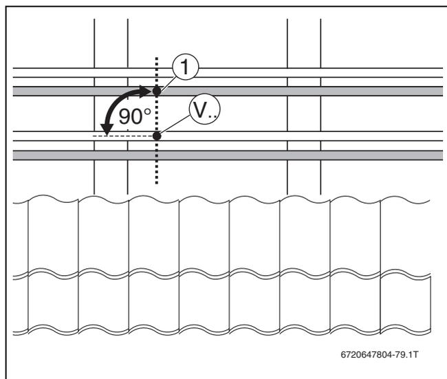
Fig. 43 Transferring reference points
