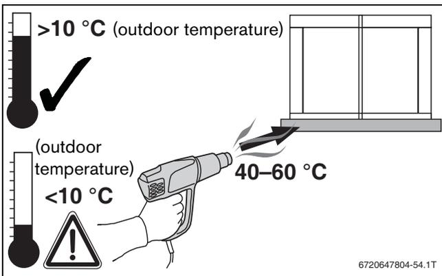
Fig. 84 Heating up the lead flashing at low outdoor temperatures
