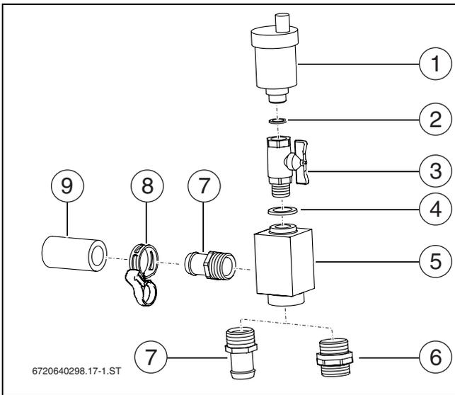
Fig. 93 Standard delivery, air vent valve set
