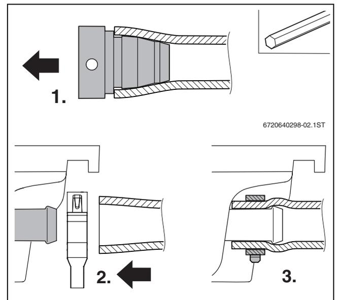
Fig. 31 Installation of the solar hose
