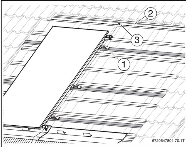
Fig. 56 Installation position of the top joiner for portrait collectors
