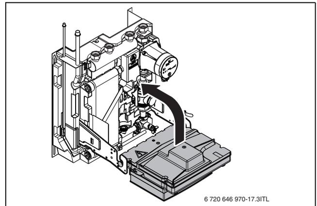
Fig. 26 Reposition the hybrid control module
