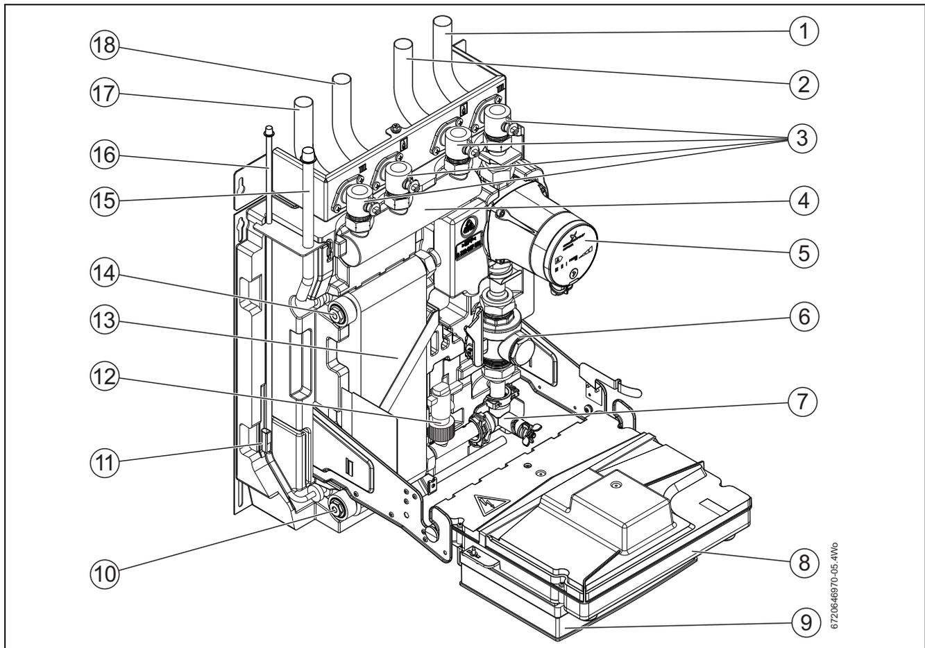
Fig. 11 Main components of the hybrid manager
