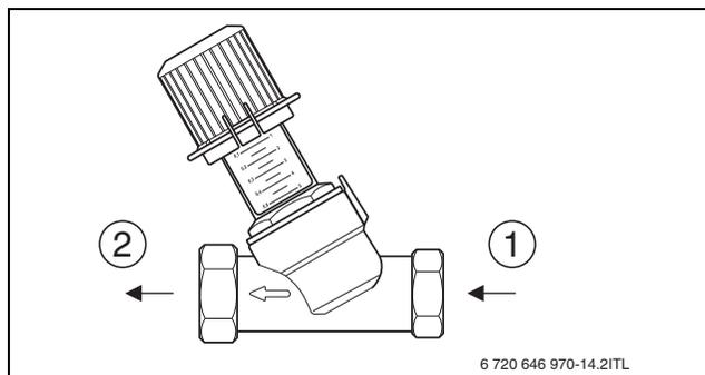
Fig. 22 Mounting the bypass valve in flow direction
