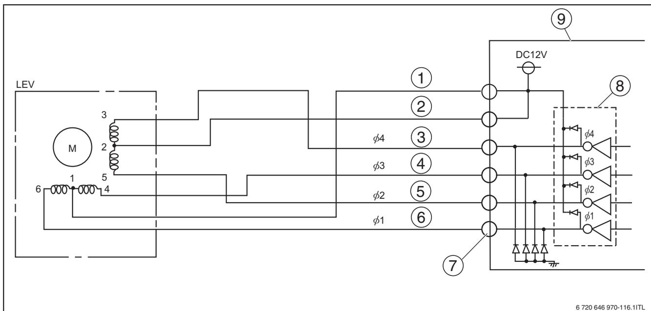
Fig. 65 Wiring diagram, linear expansion valves LE
