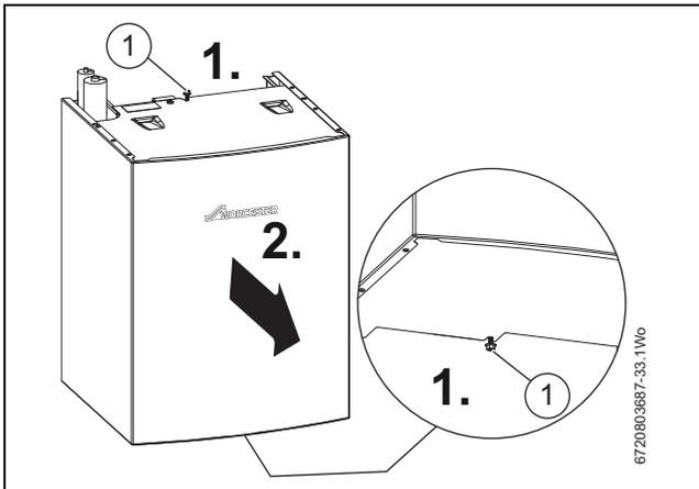
Fig. 23 Casing removal
