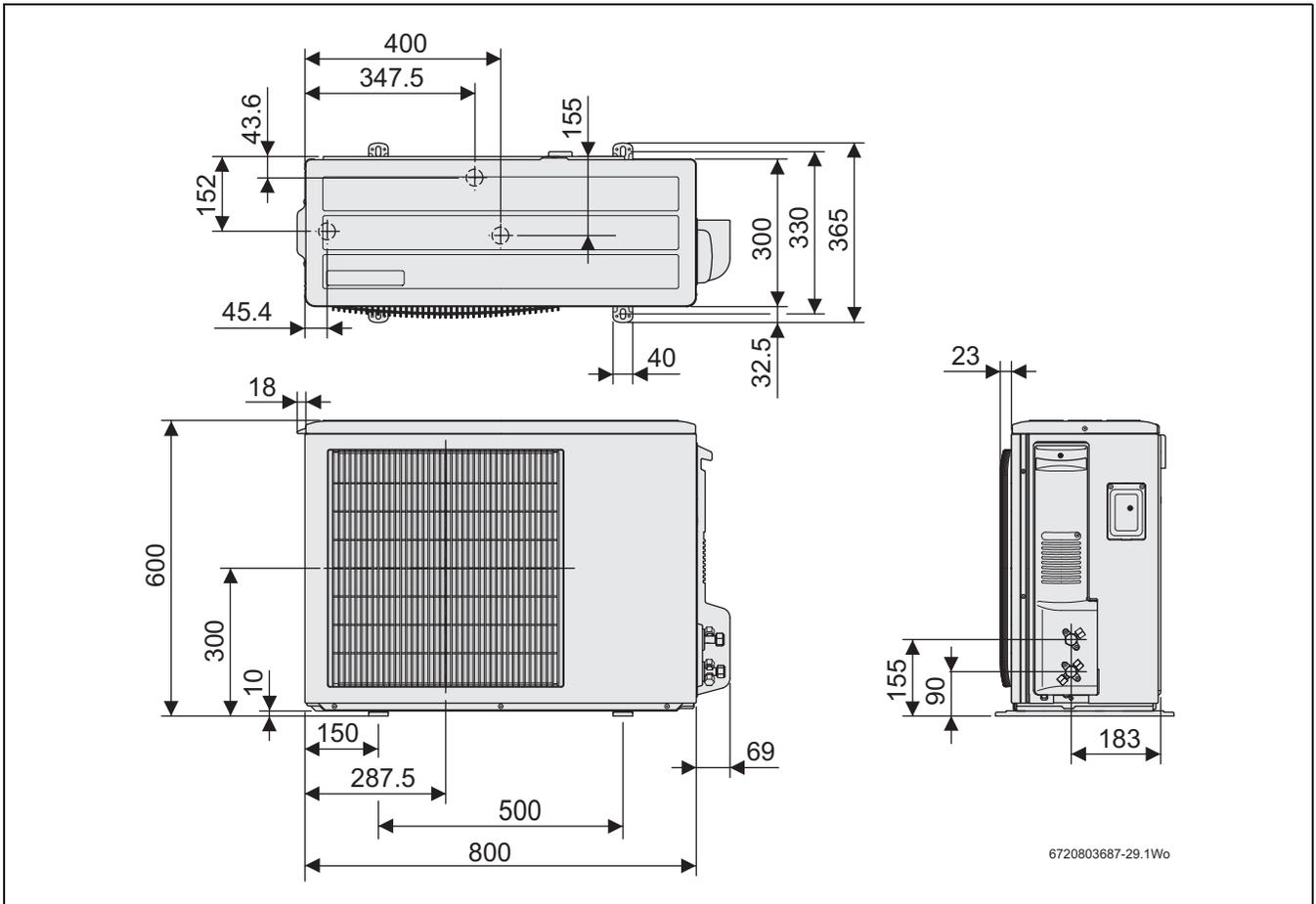
Fig. 15 Dimensions of external unit
