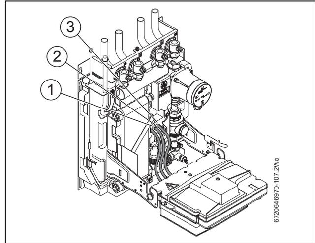
Fig. 46 Cable guide inside the hybrid manager
