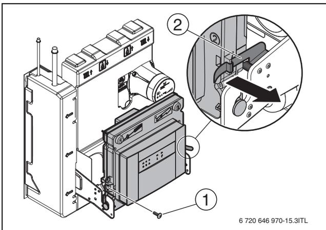
Fig. 24 Tilting the hybrid control module forward
