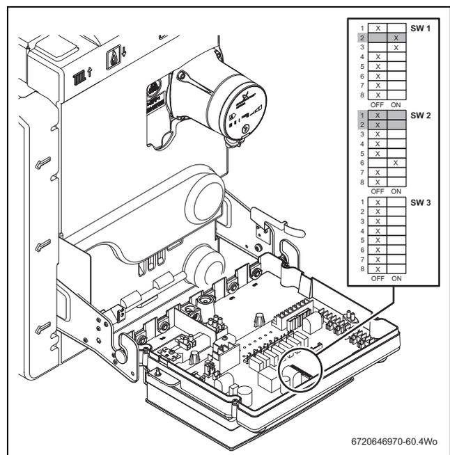
Fig. 70 DIP switches in "Pump back refrigerant" position
