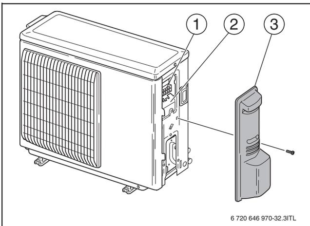
Fig. 36 Removing the service cover from the external unit
