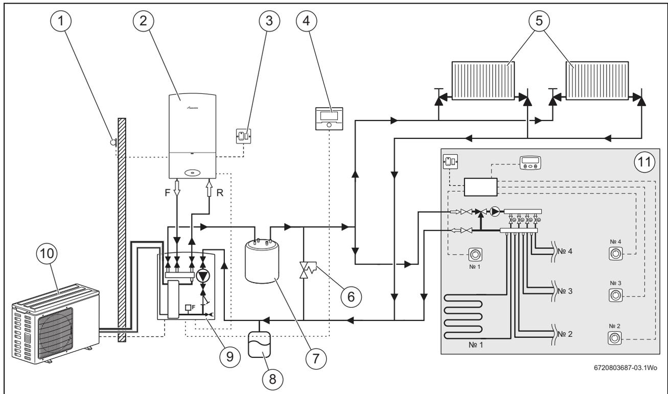
Fig. 9 System scheme with serial buffer tank, bypass valve, one unmixed heating circuit and one mixed heating circuit
