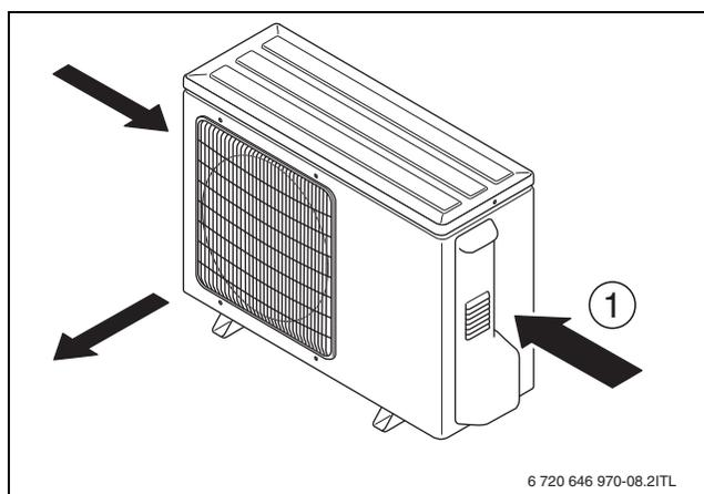
Fig. 18 Air discharge alignment
