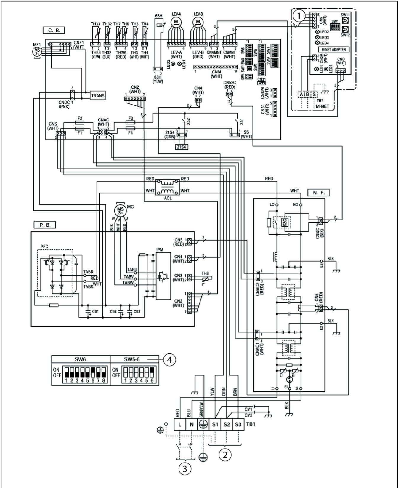
Fig. 80 Wiring to PCB in the external unit
