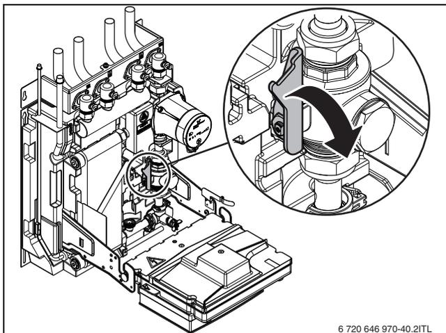
Fig. 57 Turning the filter assembly handle forward
