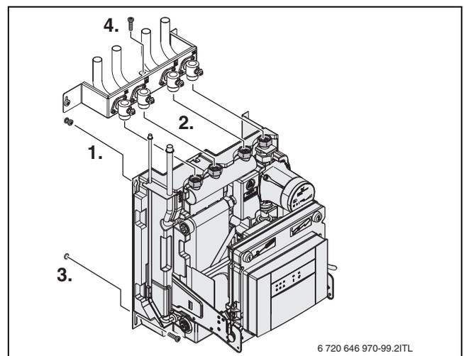
Fig. 27 Mounting the hybrid manager on the wall
