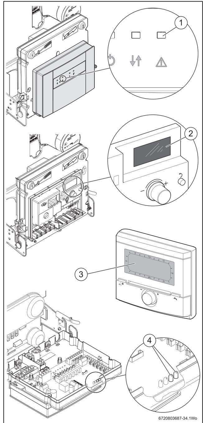
Fig. 60 Overview internal hybrid components fault indicators locations
