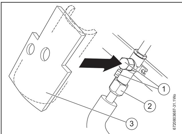
Fig. 33 Insulating material, shut-off valve and valve caps
