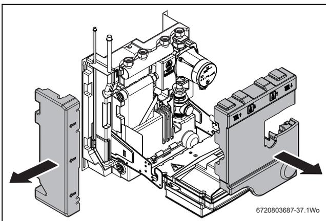
Fig. 25 Remove insulation from the hybrid manager
