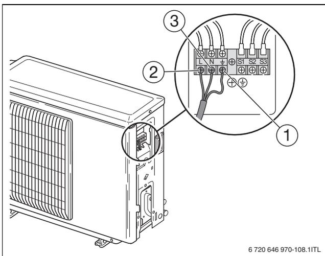
Fig. 37 Power supply to the external unit
