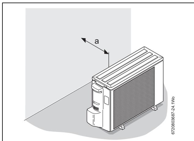
Fig. 17 Orientation towards a wall (windy location)
