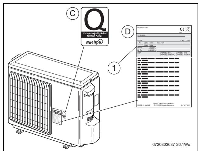
Fig. 2 Data plate on the external unit
