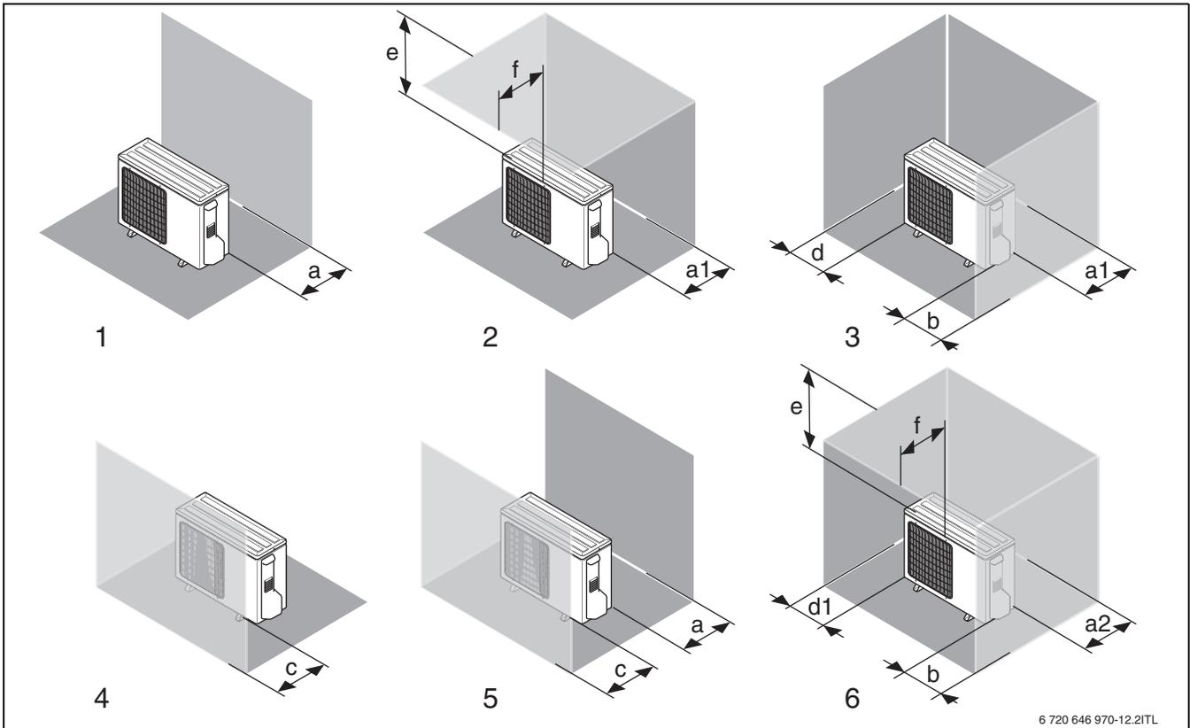
Fig. 19 Minimum clearances for specific installation situations
