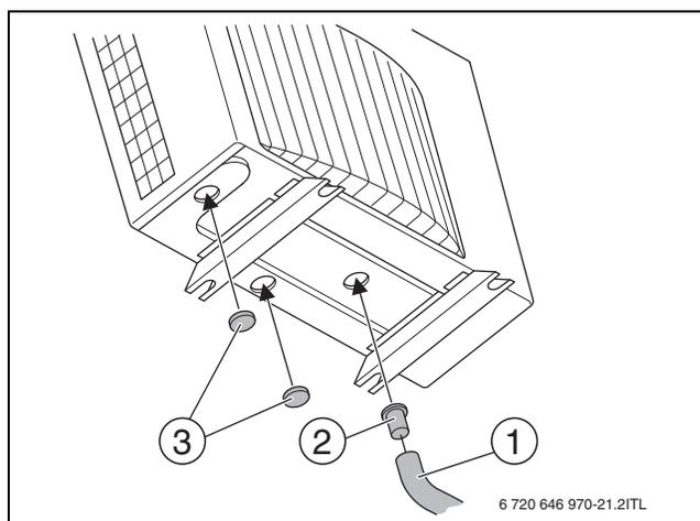
Fig. 29 Fitting the condensate drain
