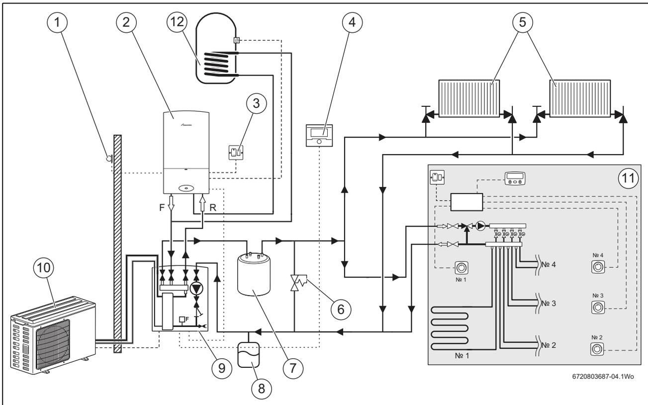
Fig. 10 System scheme with serial buffer tank and one unmixed heating circuit
