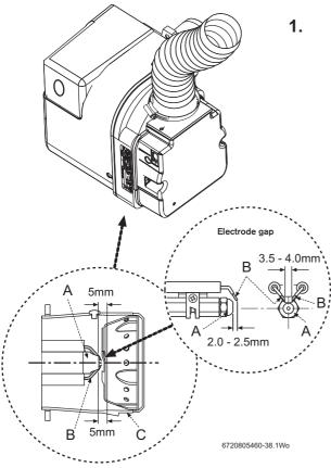
Fig. 43 Nozzle and electrode alignment
