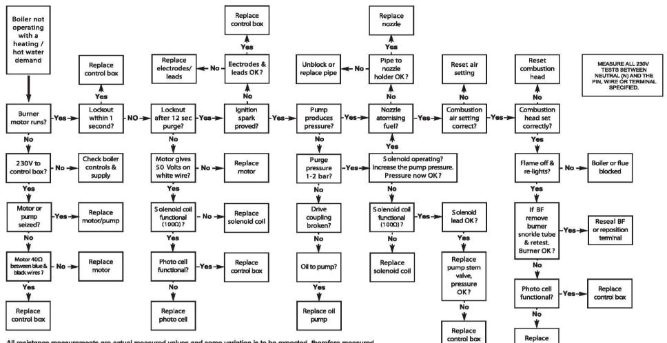
All resistance measurements are actual measured values and some variation is to be expected, therefore measured values should be similar to but not necessarily identical to the given values.
