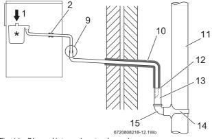
Fig. 11 Disposal into a rainwater down pipe
