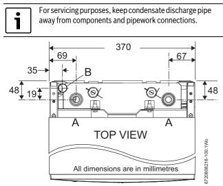
Fig. 23 Top view of Regular boiler pipe connections
