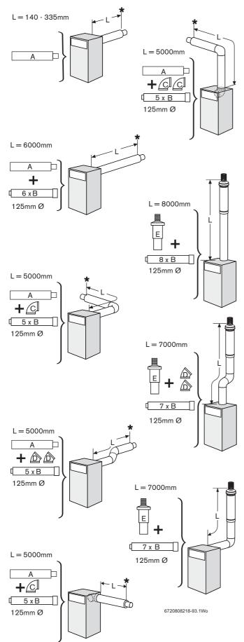
Figure 21 shows the components used and the maximum flue length (L) for each flue configuration.
