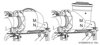
Fig. 33 Elbow retaining bracket
