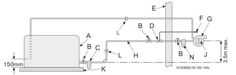
Maximum pipe run for double pipe sub-gravity fed system
