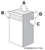
Fig. 32 Flue outlet options
