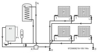
Fig. 7 System boiler system layout
