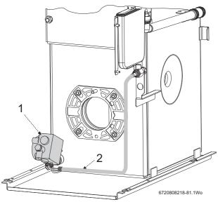
Fig. 82 Oil pump and hose detail
