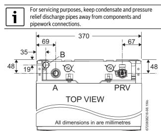
Fig. 25 Top view of System boiler pipe connections
