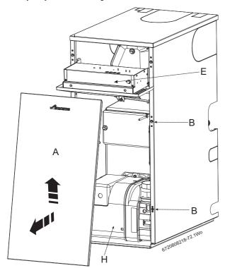
Fig. 69 Access to internal components
