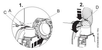
Fig. 45 Refitting the burner
