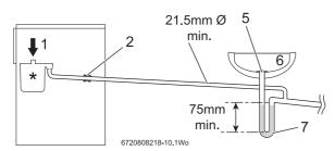
Fig. 9 Disposal to a waste pipe
