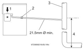
Fig. 8 Disposal to a soil vent stack
