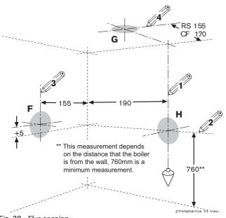
Fig. 28 Flue opening
