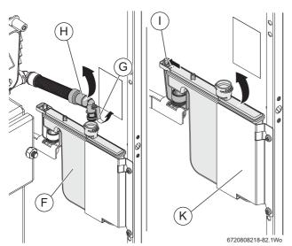
Fig. 79 Condensate trap removal
