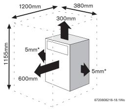
Fig. 18 Maintenance and repair clearances
