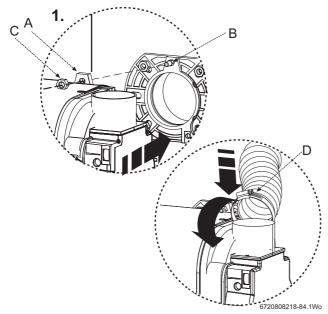
Fig. 81 Refitting the burner
