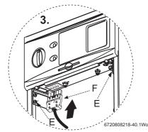
Fig. 46 Refitting the control panel
