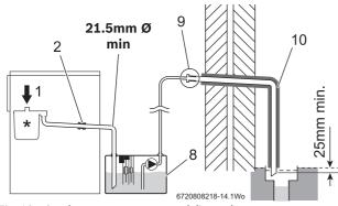
Fig. 13 Condensate pump to external disposal
