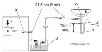
Fig. 10 Disposal via a condensate pump
