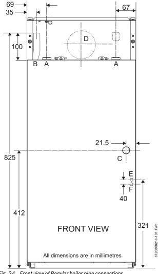
Fig. 24 Front view of Regular boiler pipe connections
