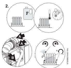
3. Drain (B) and thoroughly flush the system to remove the flushing agent and debris.
