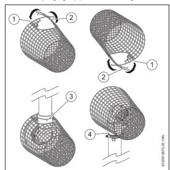
Fig. 37 Fitting terminal guard
