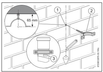
Fig. 32 Support clamp fitting
