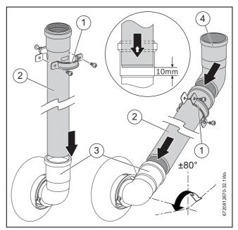
Fig. 34 Plume extension fitting
