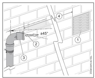
Fig. 38 Plume direction conditions
