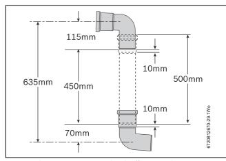
Fig. 31 Plume management 90° bends offset example
