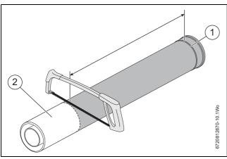
Fig. 12 Cutting an extension tube
