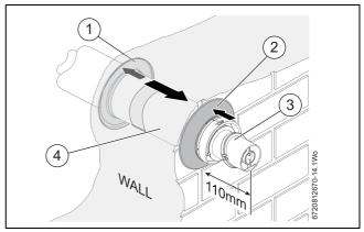
Fig. 14 Telescopic flue through the wall
