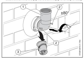
Fig. 33 Plume management terminal bend
