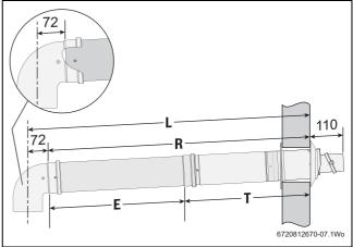
Fig. 6 Flue length determination (extended flue example)
