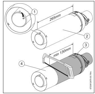
Fig. 11 Shortening the terminal assembly
