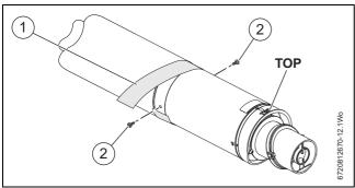
Fig. 13 Setting the telescopic flue length
