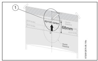
Fig. 5 Adjusted 60/100mm flue exit hole
