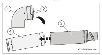
Fig. 10 Separating elbow from telescopic flue
