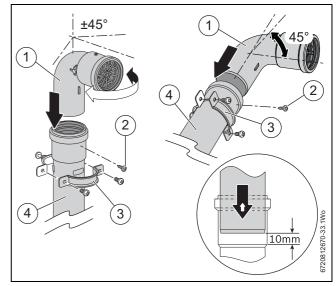
Fig. 35 Fitting the discharge elbow
