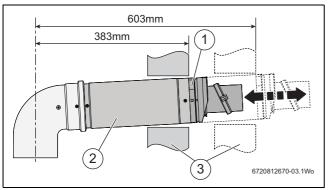
Fig. 9 Standard telescopic flue lengths
