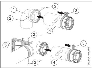
Fig. 17 Elbow connection examples (90° bend)
