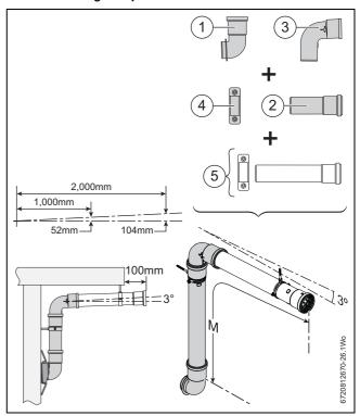
Fig. 28 Extended under a balcony/overhang option
