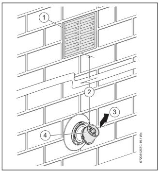
Fig. 20 Plume redirect distance to opening
