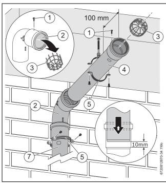
Fig. 36 Fitting extension under balcony/overhang
