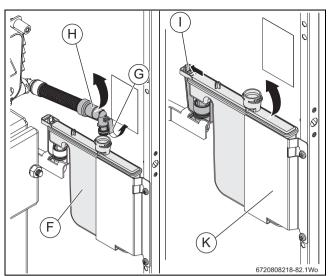
Fig. 75 Condensate trap detail
