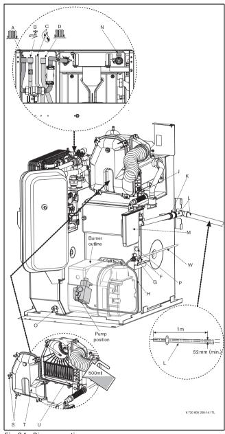
Fig. 34 Pipe connections
