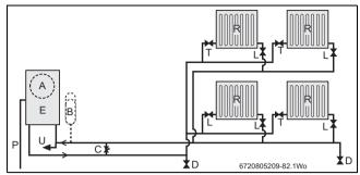
Fig. 8 Regular boiler, open vent system layout
