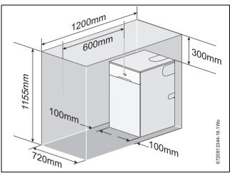
Fig. 19 Installation clearances
