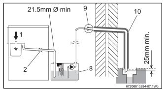
Fig. 16 Condensate pump to external disposal
