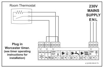
Fig. 42 Room Thermostat and Plug In Twin Channel Programmer
