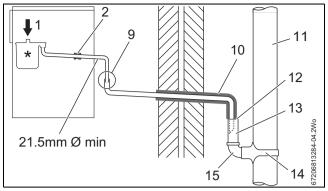
Fig. 14 Disposal into a rainwater down pipe
