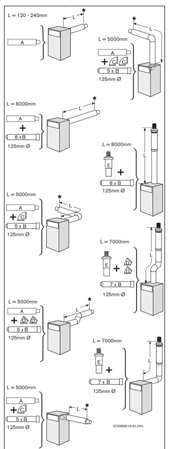
Fig. 24 Room seal ed flue options
