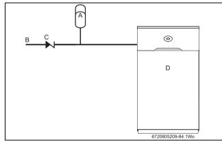
Fig. 3 Mains expansion vessel
