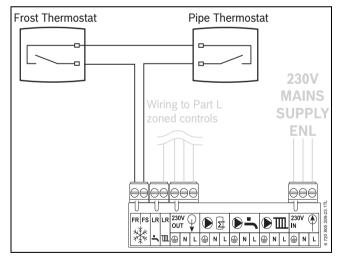
Fig. 43 Optional External 230 V AC Frost Stat Connection for protection of system pipework in unheated air space
