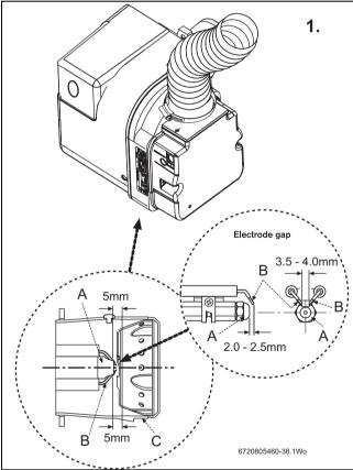
Fig. 35 Nozzle and electrode alignment
