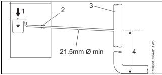
Fig. 11 Disposal to a soil vent stack
