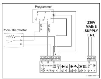
Fig. 41 External 230 V Twin Channel Programmer and Room Thermostat
