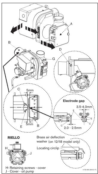
Fig. 73 Burner detail
