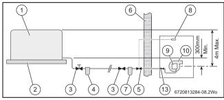
Fig. 4 Single pipe feed
