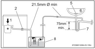
Fig. 13 Disposal via a condensate pump
