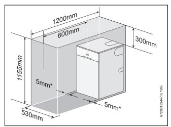
Fig. 21 Maintenance and repair clearances
