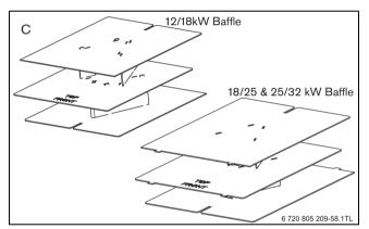
Fig. 77 Baffle arrangement
