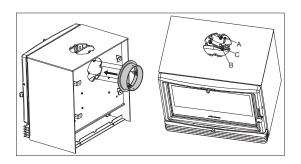
Attach the flue cover plate to the top of the stove with the four nuts you previously removed.
