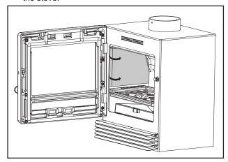
3. Rotate the end of the panel closest to you towards the door. Note: The back of the panel is angled to allow removal. When replacing the panels make sure the angled edge is in the same position as when removed.
