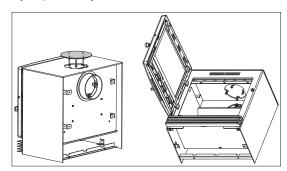
Reattach the heat shield to the back of the stove using the four 1/4-20 x 1/2 self-tapping screws that were previously removed.
