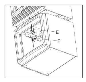
Align the holes of heat shield and stove. Insert three (3) G
