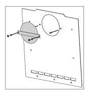
4. Remove the four nuts that are holding on the flue cover plate.
