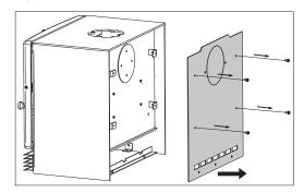
Remove the two 1/4-20 nut that are holding the heat shield cover plate on.
