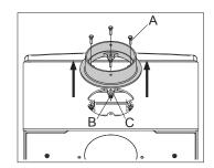
2. Remove the four 1/4-20 x 1/2 self-tapping screws that are holding the heat shield on.
