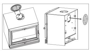
Attach the flue collar with four (A) bolts, Four (B) nuts, and four (C) washers.
