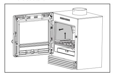
Lift up and pull the vermiculite side panel toward the front of the stove.
