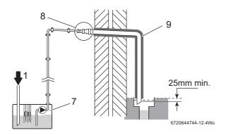
Fig. 16 Condensate pump to external disposal
