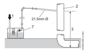
Fig. 12 Condensate pump disposal
