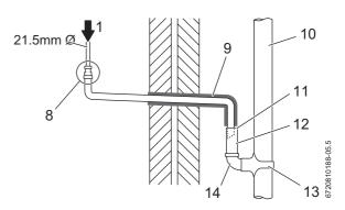
Fig. 13 Disposal into a rainwater down pipe
