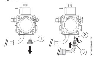
Fig. 34 Converting to double pipe system
