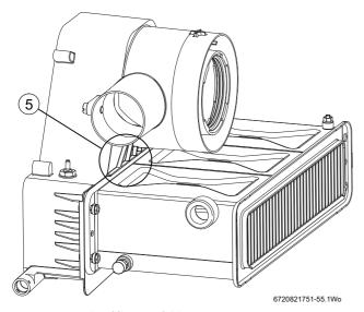
Fig. 55 Locate lip of flue manifold
