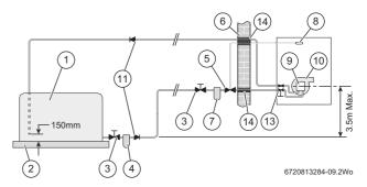
Fig. 4 Double pipe feed
