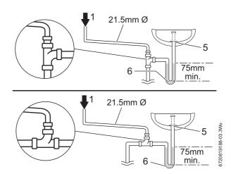
Fig. 11 Disposal to a waste pipe
