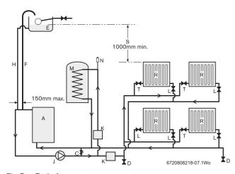
Fig. 7 Typical open vent system
