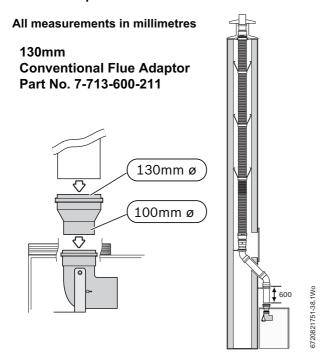
Fig. 23 Conventional Flue adapter information
