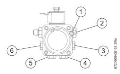
Fig. 62 Oil pump ports/connections
