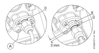
Fig. 45 RDB 3.2 BX combustion head adjustment
