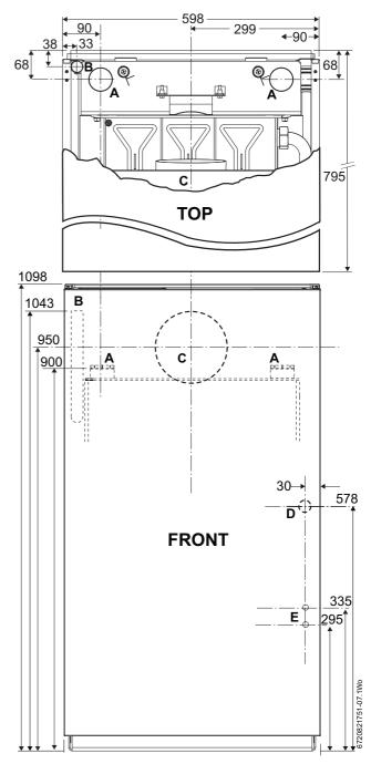
Fig. 27 Pipework position
