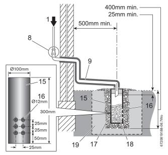
Fig. 17 Discharge to a soakaway
