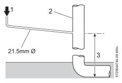
Fig. 10 Disposal to soil vent stack
