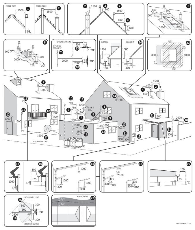
Fig. 22 Flue terminal positions
