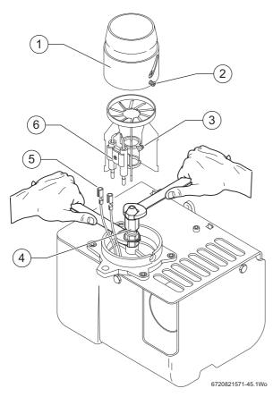
Fig. 60 Riello RDB 3.2 BT maintenance position
