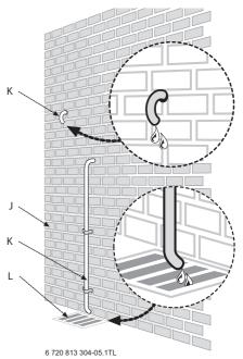
Fig. 18 Pressure relief pipe work
