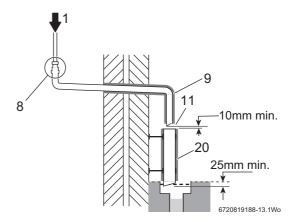
Fig. 15 External disposal with an air break
