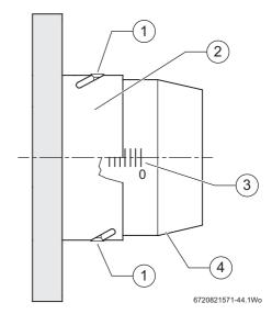
Fig. 46 RDB 3.2 BT combustion head adjustment
