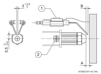
Fig. 44 RDB 3.2 BT electrode settings
