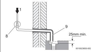
Fig. 36 Disposal to open drain or gully
