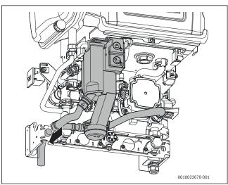
Fig. 50 Condensate connection
