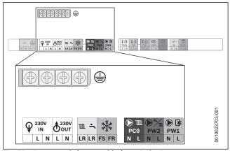
Fig. 56 Power supply (power cables) terminal strip
