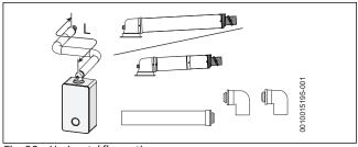
Fig. 20 Horizontal flue option
