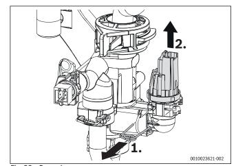
Fig. 99 Removing pressure sensor
