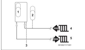
Fig. 4 Additional expansion vessel
