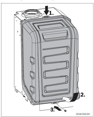
Fig. 70 Fitting the combustion casing
