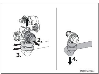
Fig. 100 Removing pressure relief valve
