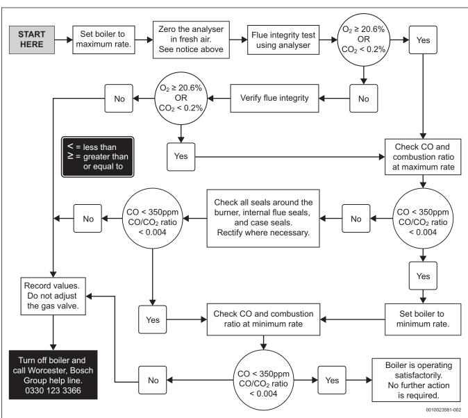
Fig. 67 Commissioning checks flow chart
