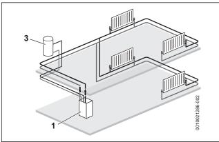
Fig. 9 Example layout - Internal diverter valve kit
