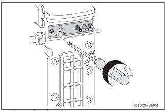
Fig. 88 Installing electrode set
