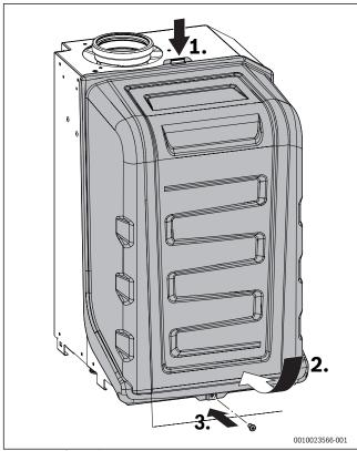
Fig. 64 Refit combustion casing
