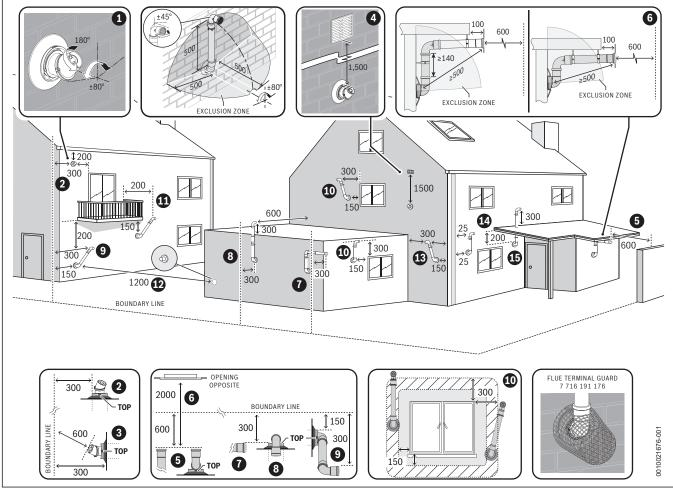
Fig. 31 Plume re-direct and plume management terminal positions
