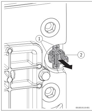
Fig. 98 Removing overheat thermostat
