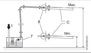
Fig. 34 Condensate pump example
