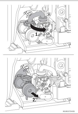
Fig. 80 Venturi removal
