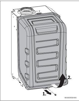
Fig. 62 Removing the combustion cover
