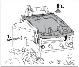
Fig. 76 Removing the burner cover
