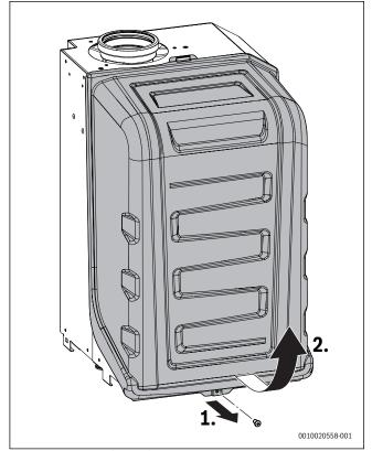
Fig. 94 Removing the combustion cover
