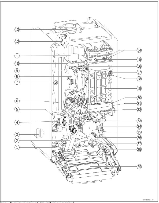
Fig. 3 Product overview System boilers, combustion cover removed
