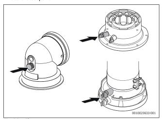
Fig. 96 Flue gas test port
