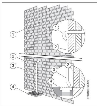
Fig. 39 Pressure relief pipe work
