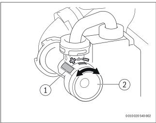
Fig. 95 Setting the adjustable venturi
