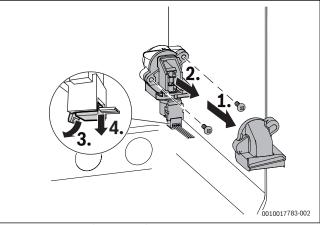
Fig. 105 Removing the 3-way valve
