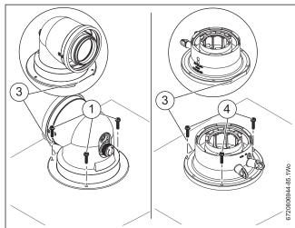
Fig. 53 Flue turret/adaptor connection
