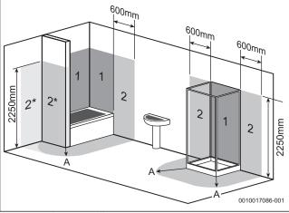
Fig. 13 Bathroom installations
