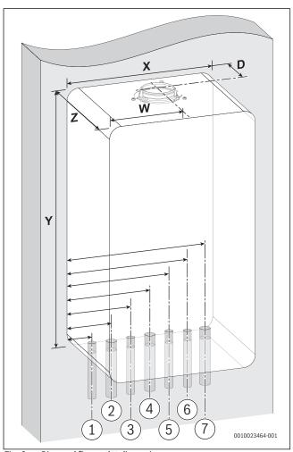
Fig. 2 Pipe and flue outlet dimensions
