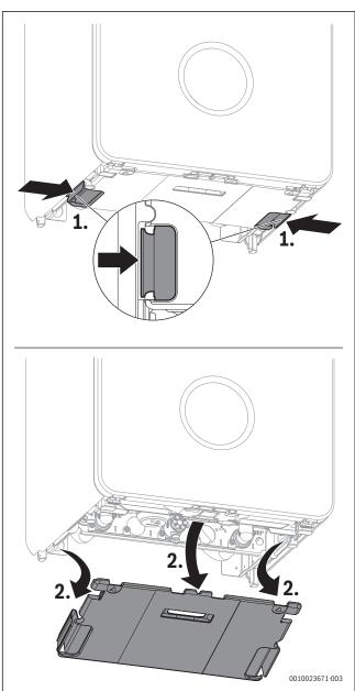
Fig. 72 Removing bottom panel
