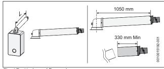
Fig. 17 Horizontal flue option
