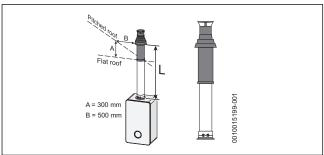
Fig. 24 Vertical flue option
