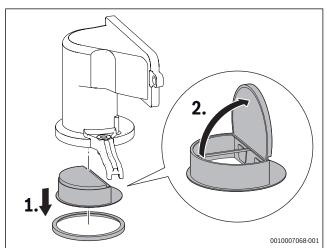
Fig. 79 Non-return valve in the air-gas manifold
