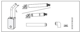
Fig. 21 Horizontal flue option
