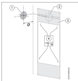
Fig. 41 Wall mounting template
