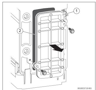
Fig. 82 Access cover removal
