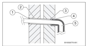
Fig. 38 Additional protection for transition through wall
