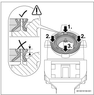
Fig. 92 Pressing on the gasket
