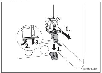
Fig. 104 Removing the motor of the 3-way valve
