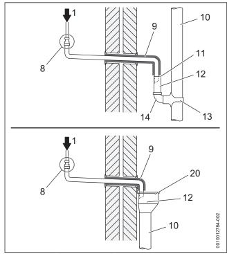
Fig. 35 Disposal into rain water down pipe
