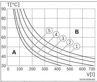
Fig. 5 Curves for the expansion vessel
