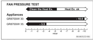
Fig. 75 Fan pressure test values
