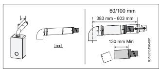
Fig. 15 Horizontal flue option
