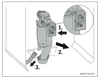
Fig. 90 Removing the condensate trap
