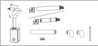
Fig. 22 Horizontal flue option
