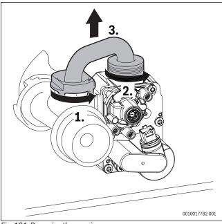
Fig. 101 Removing the gas pipe
