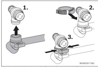
Fig. 48 Fitting the pipe on the (heating) pressure relief valve
