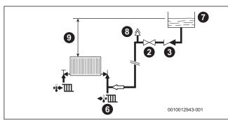
Fig. 12 Top-up tank system fill example
