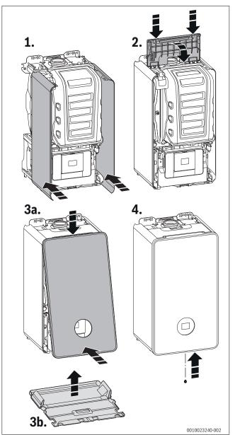
Fig. 71 Fitting the appliance casing
