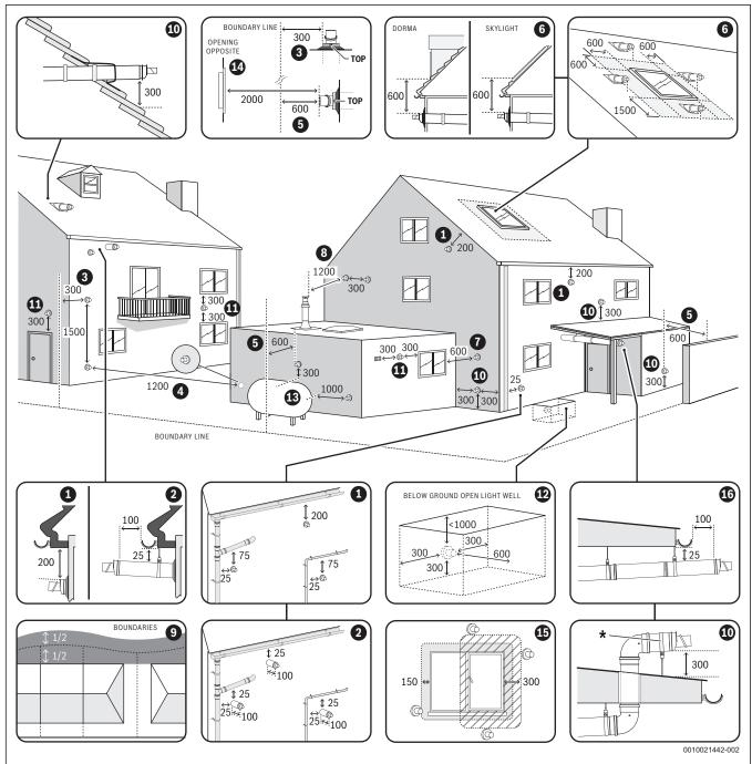
Fig. 30 Horizontal flue terminal positions
