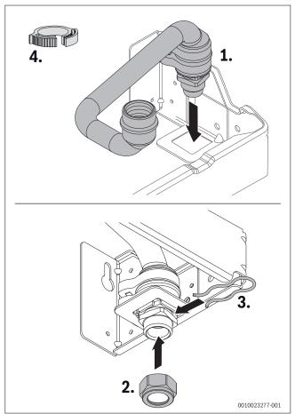
Fig. 46 Connect PRV discharge pipe
