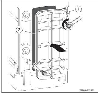
Fig. 87 Re-fitting the access cover
