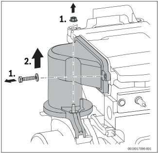
Fig. 78 Removing the air-gas manifold
