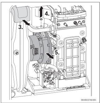
Fig. 81 Fan removal
