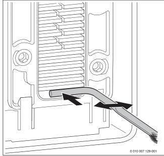
Fig. 86 Cleaning debris
