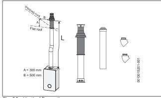
Fig. 26 Vertical flue option
