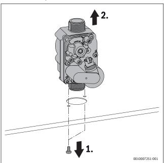
Fig. 103 Removing the gas control valve
