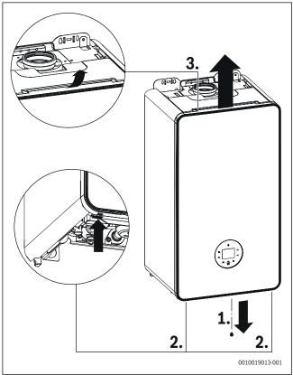
Fig. 73 Removing outer case
