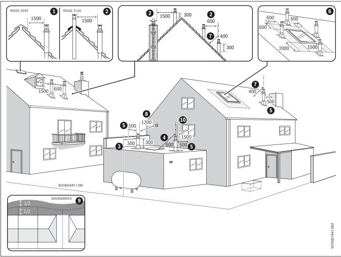
Fig. 29 Vertical flue terminal positions
