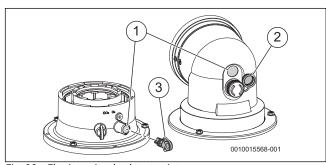
Fig. 68 Flue integrity check test point
