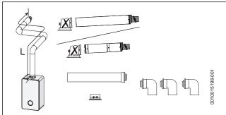
Fig. 23 Horizontal flue option
