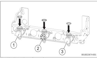
Fig. 45 Fitting the sealing washers
