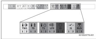
Fig. 57 Low voltage (signal cables) terminal strip
