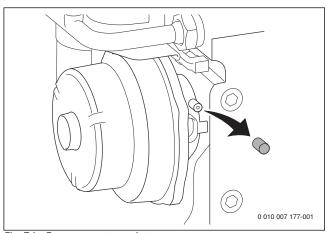
Fig. 74 Fan pressure test point
