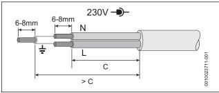
Fig. 58 Mains voltage (power cables) preparation
