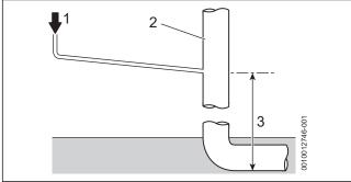
Fig. 32 Disposal to soil vent stack
