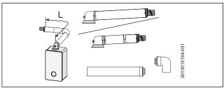
Fig. 19 Horizontal flue option
