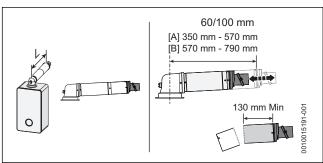
Fig. 16 Horizontal flue option
