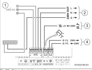
Fig. 60 External controls connections example
