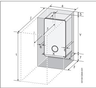
Fig. 14 Appliance minimum clearances
