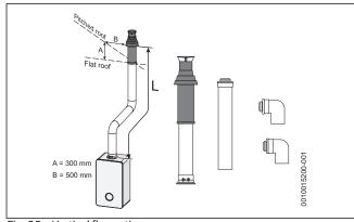
Fig. 25 Vertical flue option
