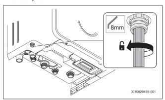
Fig. 79 Drain point
