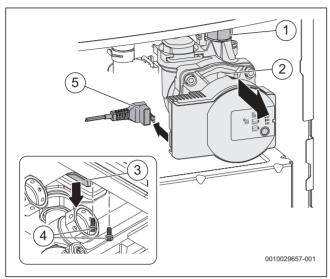
Fig. 85 Removing the pump
