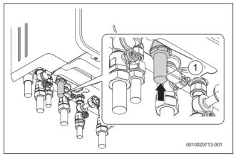
Fig. 43 Connecting to the PRV tail connection
