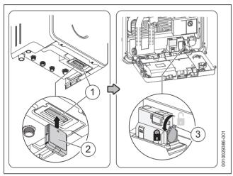
Fig. 50 Installing the Key
