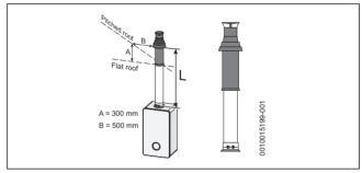
Fig. 21 Vertical flue option
