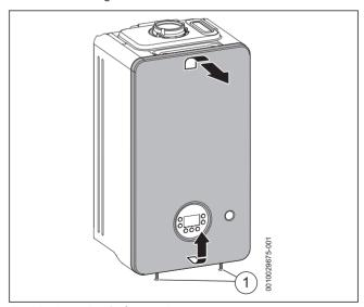
Fig. 60 Removing the front casing
