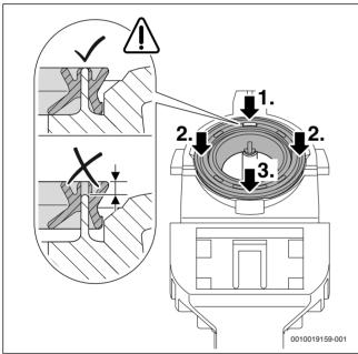
Fig. 75 Pressing on the gasket
