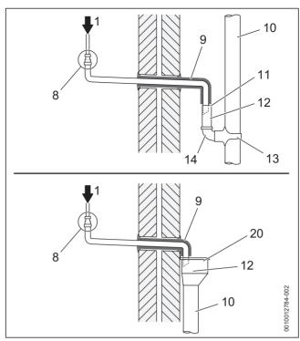
Fig. 32 Disposal into rain water down pipe
