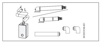
Fig. 17 Horizontal flue option
