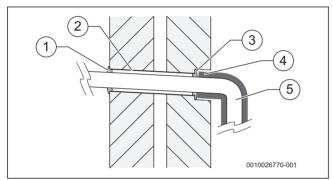
Fig. 35 Additional protection for transition through wall
