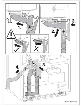
Fig. 76 Inserting the condensate trap
