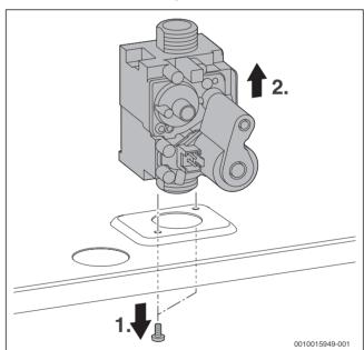
Fig. 84 Removing the gas valve
