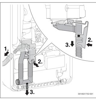
Fig. 71 Removing the condensate trap
