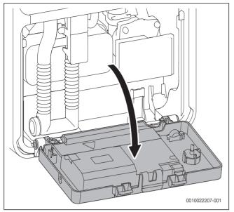
Fig. 46 Moving control panel into service position
