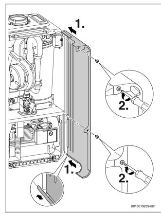
Fig. 92 Attaching the side panel
