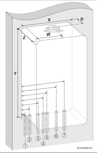
Fig. 2 Pipe and flue outlet dimensions
