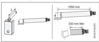
Fig. 14 Horizontal flue option
