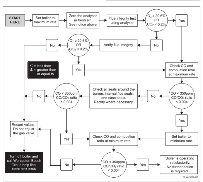
Fig. 56 Commissioning checks flow chart
