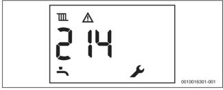
Fig. 93 Example: non-blocking fault
