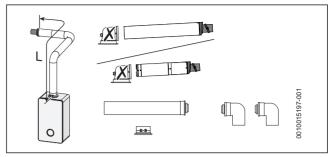
Fig. 19 Horizontal flue option
