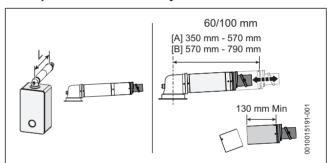
Fig. 13 Horizontal flue option
