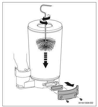
Fig. 68 Cleaning the heat exchanger
