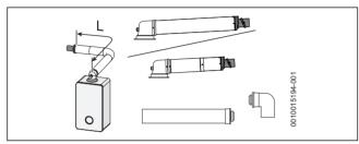
Fig. 16 Horizontal flue option
