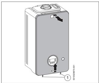
Fig. 40 Removing the front casing
