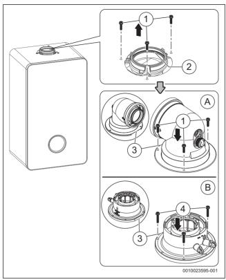
Fig. 45 Flue turret/adaptor connection
