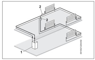
Fig. 7 Separated heating zones
