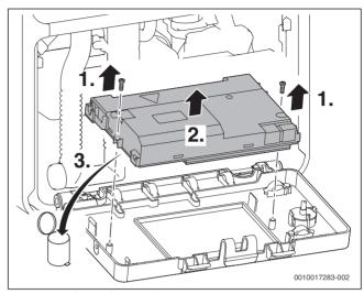
Fig. 90 Replacing the control unit
