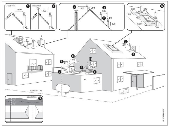
Fig. 26 Vertical flue terminal positions
