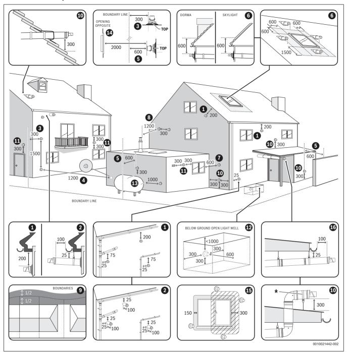
Fig. 27 Horizontal flue terminal positions
