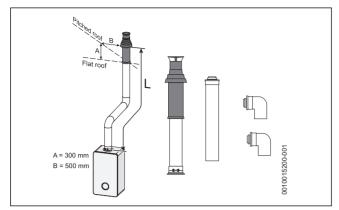
Fig. 22 Vertical flue option
