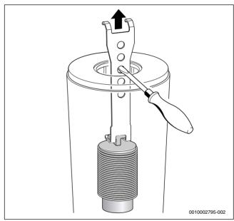
Fig. 67 Removing the bottom baffle
