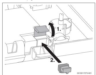
Fig. 91 Inserting the code plug
