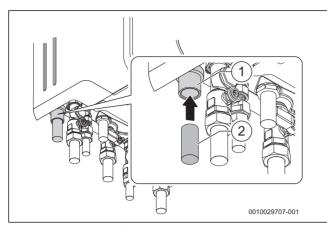
Fig. 42 Connecting to the condensate outlet connection
