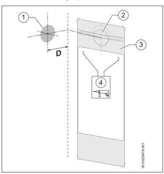
Fig. 37 Wall mounting template
