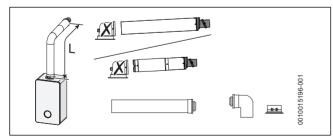
Fig. 18 Horizontal flue option
