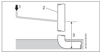
Fig. 29 Disposal to soil vent stack
