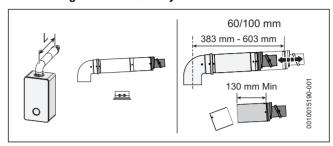
Fig. 12 Horizontal flue option
