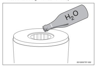
Fig. 70 Purge the heat exchanger with water
