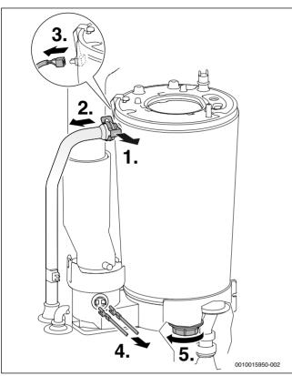
Fig. 88 Detach the flow pipe and disconnect the cable
