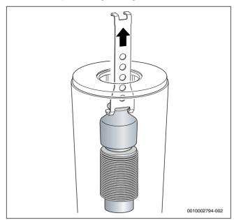
Fig. 66 Remove the top baffle
