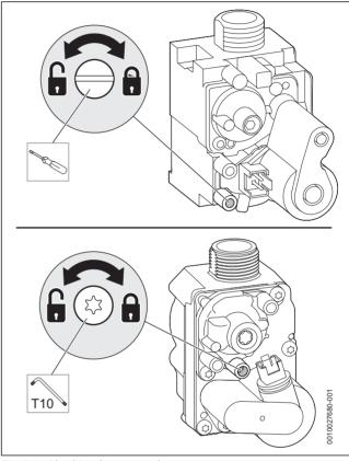
Fig. 54 Checking the gas supply pressure
