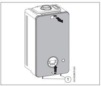
Fig. 78 Removing the front casing
