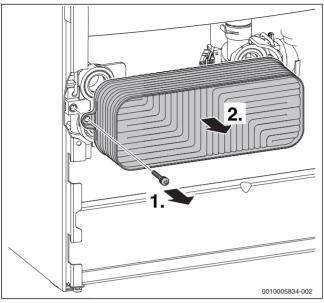
Fig. 82 Removing the plate heat exchanger
