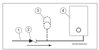
Fig. 9 Mini expansion vessel location
