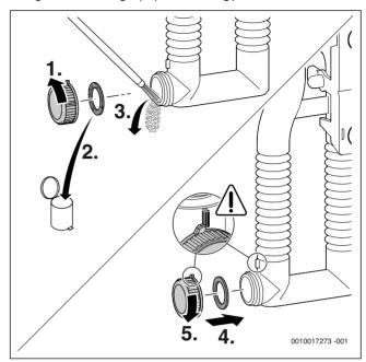
Fig. 72 Cleaning the condensate trap
