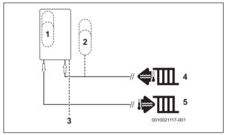
Fig. 4 Additional expansion vessel
