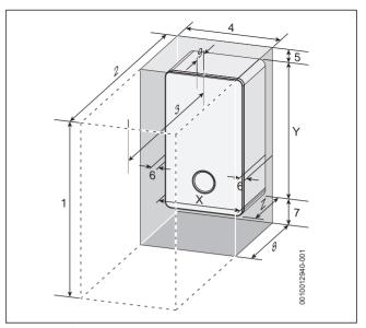
Fig. 11 Appliance minimum clearances
