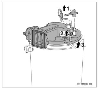
Fig. 63 Remove the burner cover
