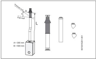
Fig. 23 Vertical flue option
