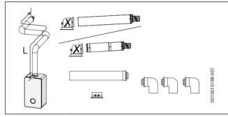
Fig. 20 Horizontal flue option
