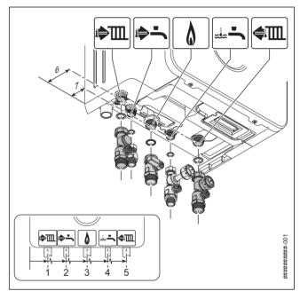
Fig. 38 Fitting the connection sets
