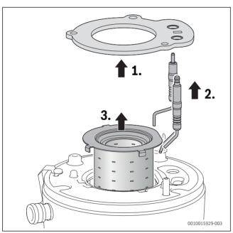
Fig. 65 Removing the burner
