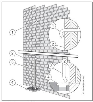
Fig. 36 Pressure relief pipe work
