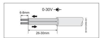
Fig. 49 Low voltage (signal cables) preparation
