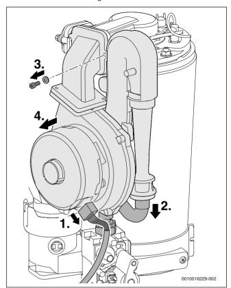
Fig. 62 Removing the fan with mixing device
