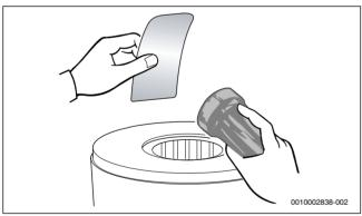
Fig. 69 Checking the heat exchanger for residue
