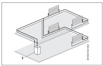
Fig. 6 Single central heating circuit example
