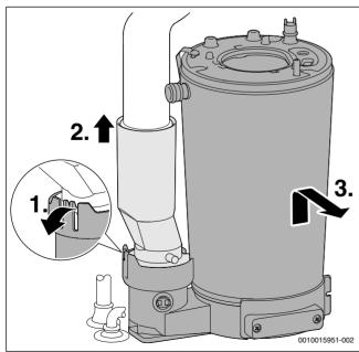
Fig. 89 Removing the heat exchanger
