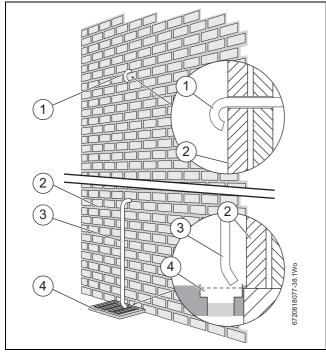
Fig. 39 Pressure relief pipework
