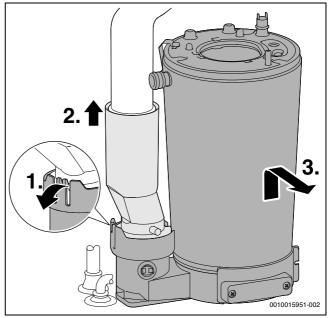
Fig. 100 Removing the heat exchanger
