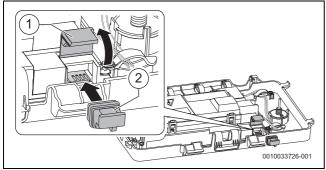
Fig. 102 Inserting the code plug
