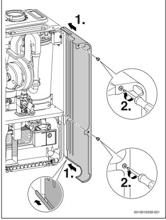
Fig. 104 Attaching the side panel
