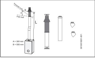
Fig. 25 Vertical flue option
