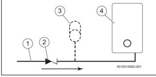
Fig. 9 Mini expansion vessel location
