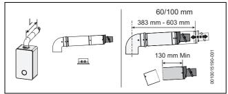
Fig. 14 Horizontal flue option
