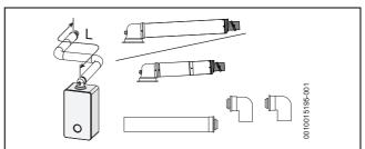
Fig. 19 Horizontal flue option
