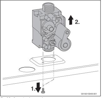
Fig. 95 Removing the gas valve
