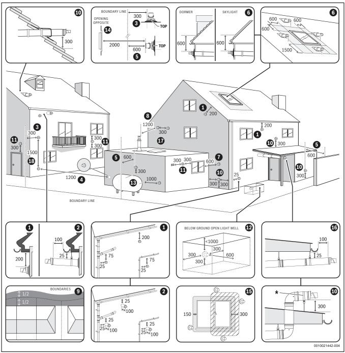
Fig. 29 Horizontal flue terminal positions
