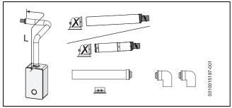
Fig. 21 Horizontal flue option
