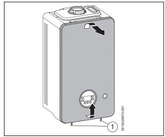
Fig. 89 Removing the front casing
