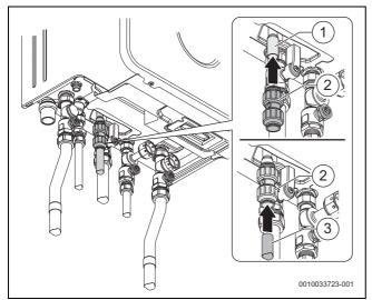
Fig. 45 Connecting to the PRV tail connection
