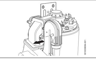
Fig. 72 Test nipple at the mixing device
