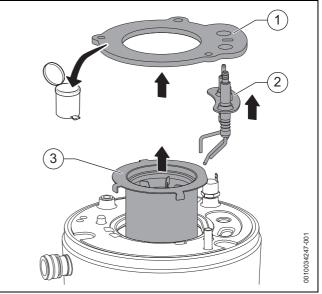
Fig. 76 Removing the burner
