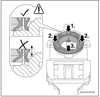
Fig. 85 Pressing on the gasket
