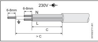
Fig. 56 Mains voltage (power cables) preparation Low voltage (signal cables), example  $\rightarrow$  figure 57
