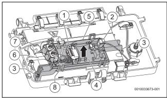
Fig. 103 Replacing the Control box housing with PCB
