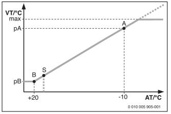
Fig. 106 Heating curve
