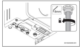
Fig. 90 Drain point
