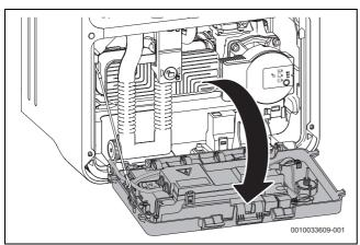
Fig. 51 Moving control panel into service position
