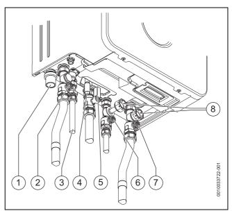
Fig. 44 Connections on the gas and water side
