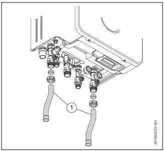
Fig. 43 CH pipe tails fitting
