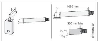
Fig. 16 Horizontal flue option
