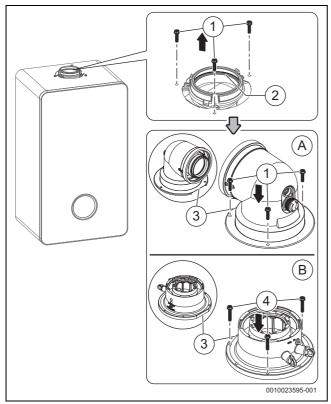
Fig. 49 Flue turret/adaptor connection
