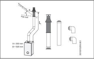
Fig. 24 Vertical flue option
