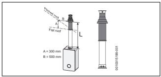
Fig. 23 Vertical flue option
