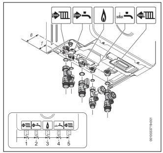
Fig. 42 Fitting the connection sets (for orientation reference)
