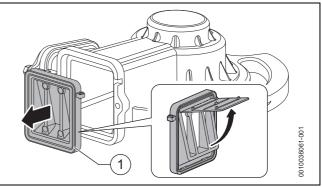
*Fig.* 75 Non-return valve (bearing plate) in the mixing unit Refer to figure 76.
