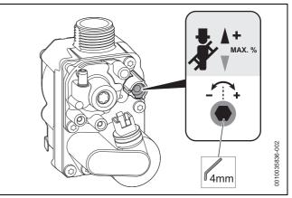
Fig. 88 Setting the CO<sub>2</sub> content
