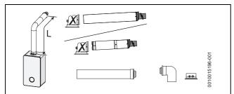
Fig. 20 Horizontal flue option
