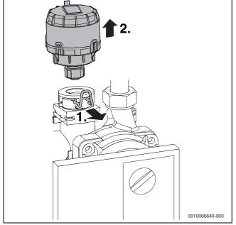
Fig. 98 Removing the motor of the diverter valve
