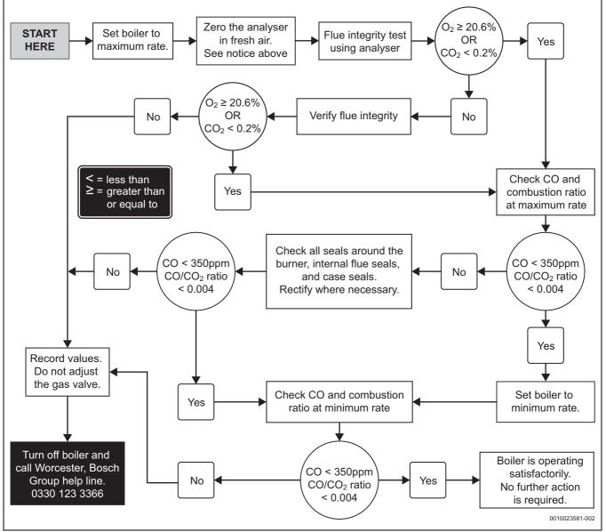
*Fig.* 66 *Commissioning checks flow chart*
