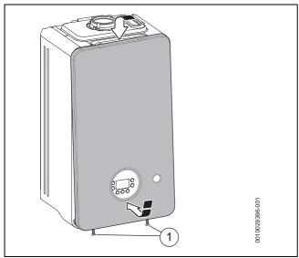
Fig. 69 Fitting the front panel
