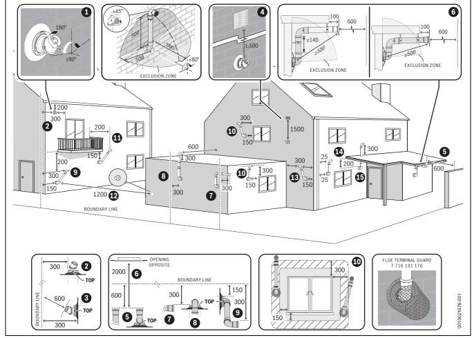
Fig. 30 Plume re-direct and plume management terminal positions
