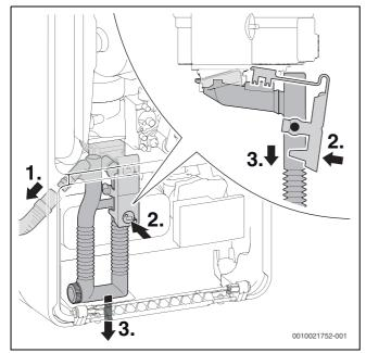
Fig. 81 Removing the condensate trap
