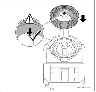
Fig. 84 Aligning the gasket with the condensate trap
