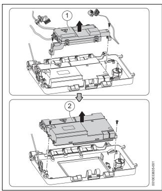
Fig. 101 Replacing the control unit
