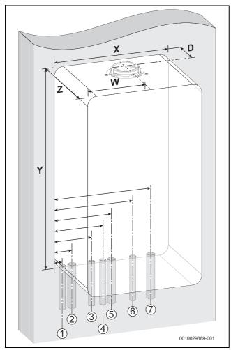
*Fig. 2 Pipe and flue outlet dimensions*
