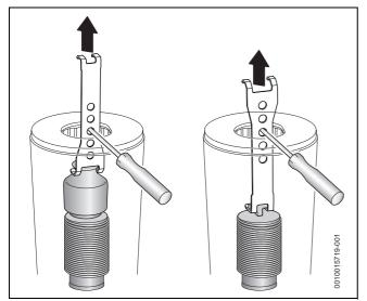
Fig. 77 Remove the top and bottom baffles
