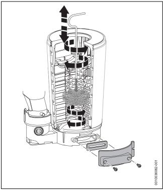
Fig. 78 Cleaning the heat exchanger
