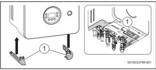
Fig. 70 Assembly direction of infills
