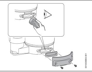
Fig. 80 Checking the heat exchanger for residue
