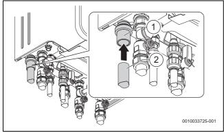
Fig. 46 Connecting to the condensate outlet connection
