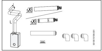
Fig. 22 Horizontal flue option
