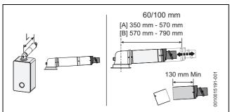
Fig. 15 Horizontal flue option
