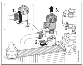
Fig. 91 Remove the pressure relief valve (heating circuit)
