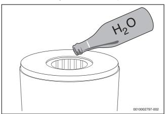
Fig. 79 Rinse the heat exchanger with water
