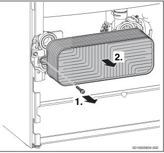
Fig. 93 Removing the plate heat exchanger
