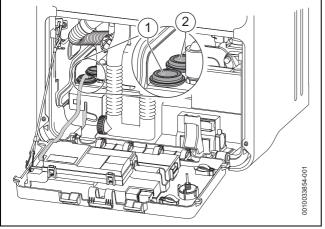
Fig. 50 Mains supply cable routing
