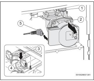
Fig. 96 Removing the pump
