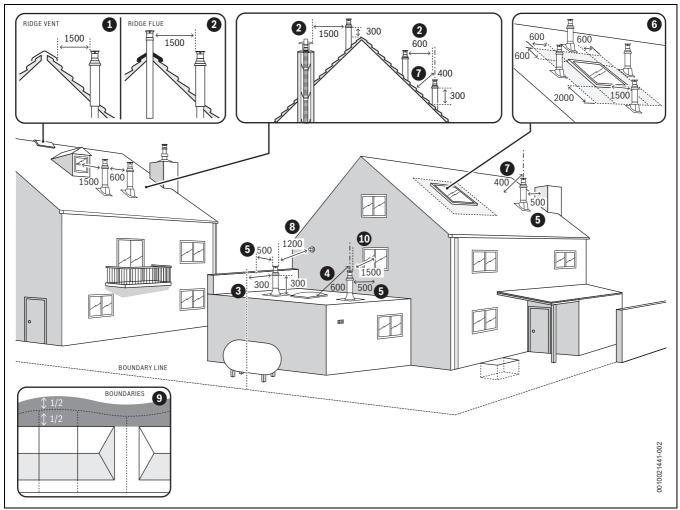
Fig. 28 Vertical flue terminal positions
