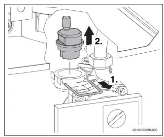
Fig. 97 Removing the automatic air vent valve
