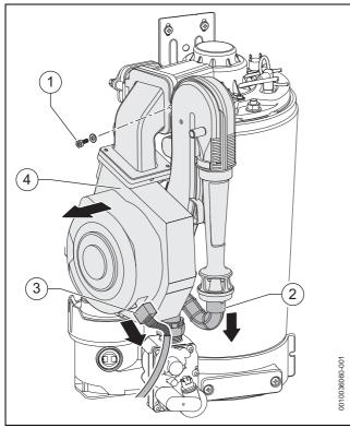
*Fig.* 73 *Removing the fan with mixing unit* Refer to figure 74.
