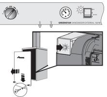
4. Boiler mode light ON, Lockout light OFF
