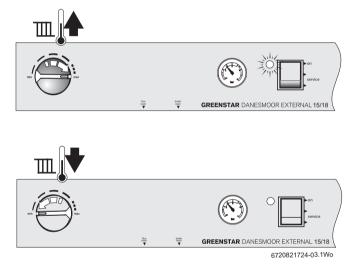
The minimum and maximum ranges of the temperature control positions are approximately 55°C to 81°C.
