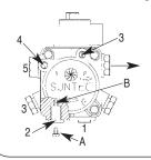
To convert to a double pipe system, remove the return port plug (2) and insert the grub screw (A) provided into the threaded hole (B). Connect flow and return pipes to (1) and (2).
