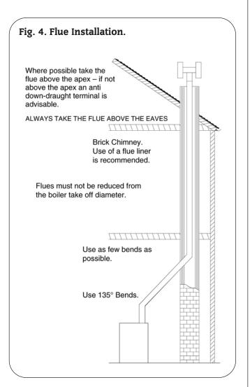
The boiler is fitted with a conventional flue locating spigot. The flue pipe fits into the spigot and should be correctly sealed with fire cement.
