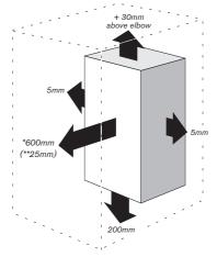
\*600mm service clearance required to a fixed surface (\*\*25mm from removable door or panel)
