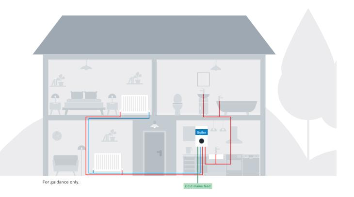
A combination (or combi) boiler powers your central heating and hot water requirements from a single compact unit.
