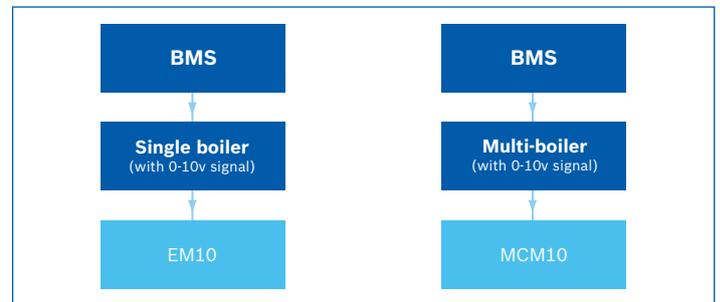
Fig. 1. Compatible BMS controls
