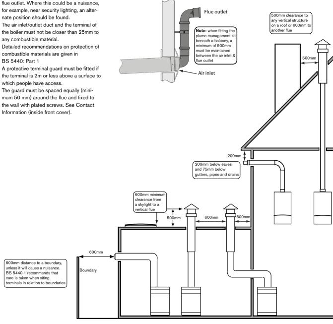
Deduct one metre off the total flue length for every 45° bend used Deduct two metres off the total flue length for every 90° bend used
