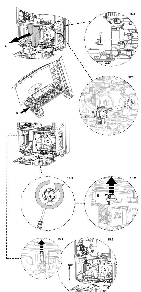
**NOTE:** Removal of the syphon assembly will give access to Auto air vent.
