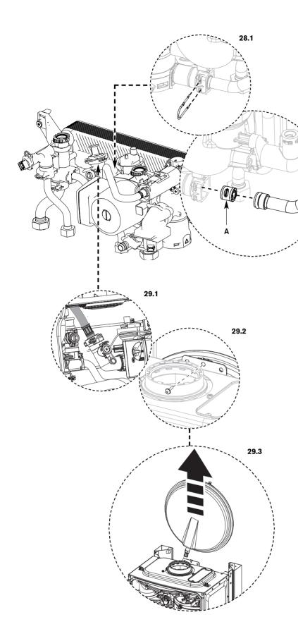
**NOTE:** Remove the Hydraulic block from the boiler (Refer to page 51).
