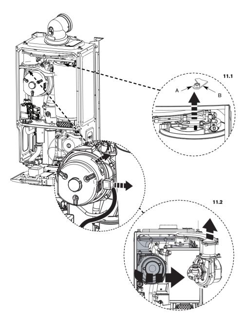
The following components require the air / gas manifold and fan assembly to be removed:
