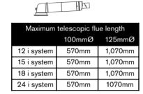
High level horizontal flue with 3x90° bends
