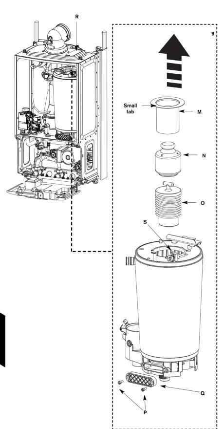
IMPORTANT: IF THE JOINT BETWEEN THE AIR/GAS MANIFOLD AND THE HEAT EXCHANGER IS DISTURBED THE SEALING GASKET MUST BE REPLACED.
