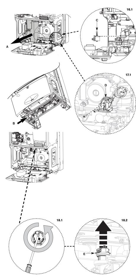
**NOTE:** Removal of the syphon assembly will give access to Auto air vent.
