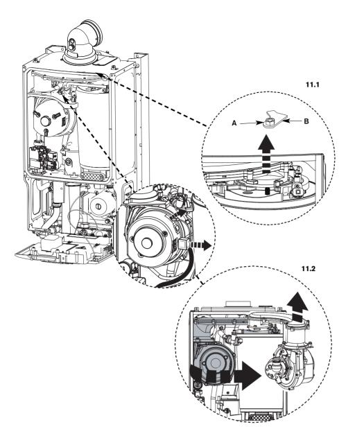
The following components require the air / gas manifold and fan assembly to be removed:
