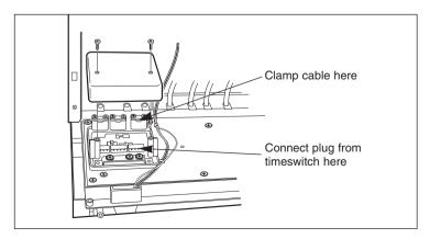
Replace the electrical box cover, splash cover and fascia bottom panel, secure the fascia using the two screws and refit the front panel
