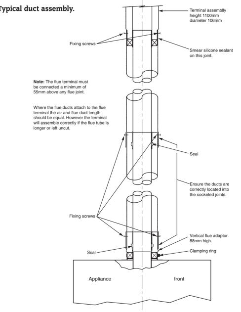
**Important:** Do not forget to fix the fire stop spacer as the assembly of the system proceeds.
