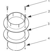
1. Flue spigot fixing screws
