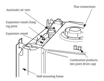
**12.1** Remove the appliance cabinet by removing the screw at the top centre of the cabinet.
