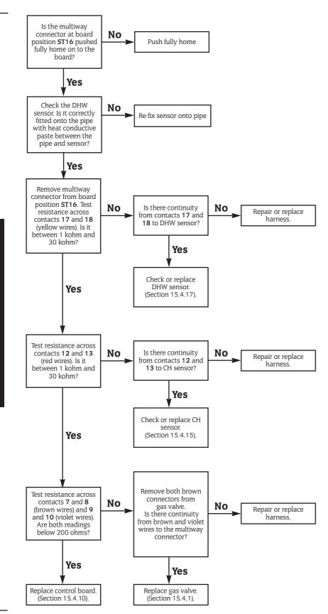
FAIL POINT I "Sensor Fault"
