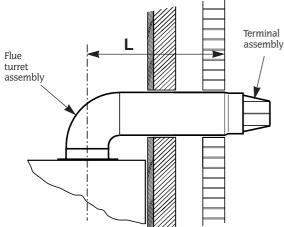
NOTE: Extension duct measurements do not include the socketed end. Unless specifically instructed the socketed end must not be removed.
