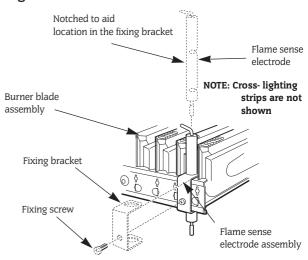
and remove the flame sensing electrode assembly. Refer to Fig 47. Ensure that the electrode is at the correct height above the burner blade.
