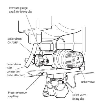
Do not omit the O-ring from the pressure capillary when fitting the replacement gauge.
