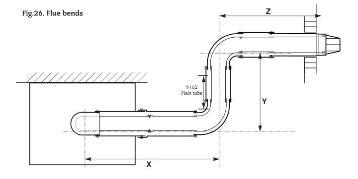
If more than two extension ducts are needed in any section to achieve the required length then the final section of the assembly must not be less than 325mm without cutting the terminal assembly.
