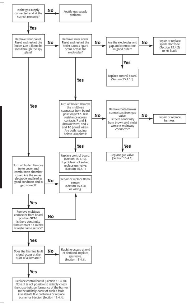
FAIL POINT H "Burner Lockout"
