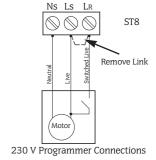
230 V room thermostat and Programmer Connections
