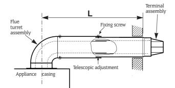
If L is greater than 725mm then extension duct kit/s will be required - each kit extends the flue by 750mm up to a maximum of 2975mm. See table below.
