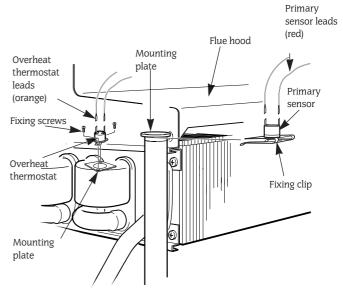
Apply a small quantity of heat transfer paste to the face of the replacement sensor.
