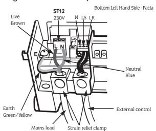
Note: When the mains ON/OFF switch on the facia is turned OFF the 2amp fuse is still live. Refer to Fig.12.
